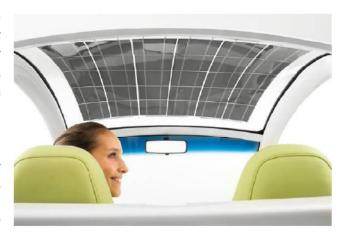
In this way, the vehicle has no need for a charging terminal, as it recovers lost solar energy rather like a rainwater collector on a roof, and recharges the batteries when the vehicle is at rest so that it can use the energy later on.
