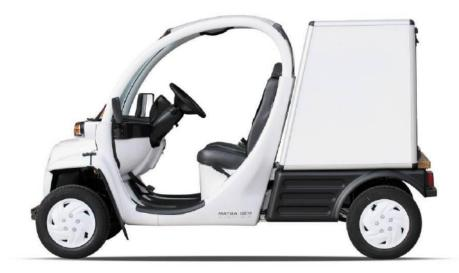
With its compact size (only 2.97 m long, 1.41 m wide, and 1.80 m high) facilitating on-board access, an exceptional load capacity for its size, and a loading surface of 1.17 m<sup>2</sup> for a load capacity of 1.2 m<sup>3</sup>, the GEM eM is an 100% green solution adapted to the constraints of deliveries in town centres.
