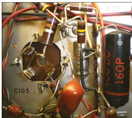
Figure 10. C107 (silver case) is located under discrete components and the black jumper.
