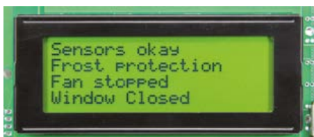
Figure 4. Some of the reports shown on the LCD module of the ventilation system.
