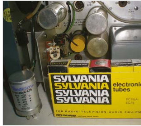
Figure 12. New C30 can capacitor and NOS 6CB6A tubes.
