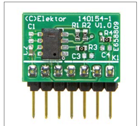
Figure 1. This adaptor board makes it a lot easier to work with the ChipCap2 sensor.
