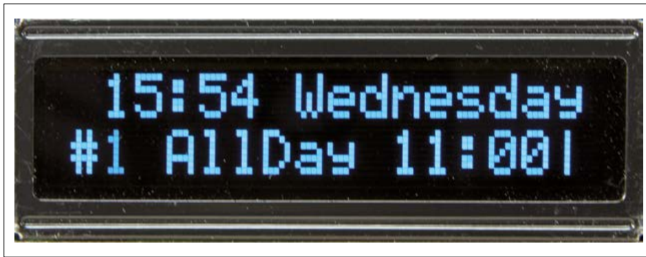
Figure 2. After pressing S1 the alarm-setting menu appears on the bottom line of the display.
