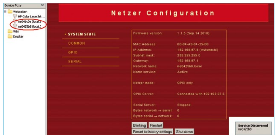
Figure 4. The 'Bonjour' browser plug-in scans the network for devices (on the left of the picture). This allows access to the module without having to know its actual IP address.
