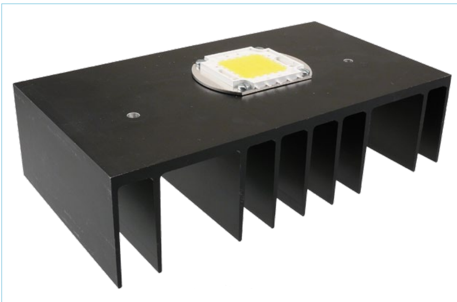
Figure 5. This LED module obviously requires cooling. Following the motto 'better safe than sorry', we drew a somewhat oversized heat sink from stock for our circuit.
