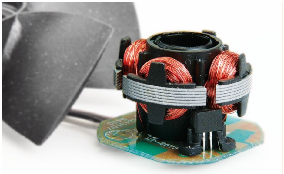
Figure 1. The secrets of a fan: two coils and a dedicated control IC.
