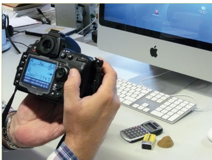
Figure 4. You can also approximate the light intensity with the aid of a digital camera and Table 2.
