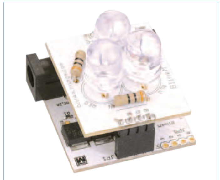
Figure 10. The mega-pixel BlinkM MaxM display is amazingly powerful, it generates a light source 1000 times brighter than a standard high-brightness LED! So it’s vital never to look directly at the light source, at risk of serious eye damage.
