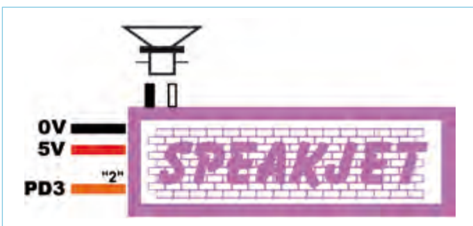
Figure 9. Connecting up the Speakjet. Note that the pin referred to as ‘2’ is the one next to the ‘TX’ pin.
