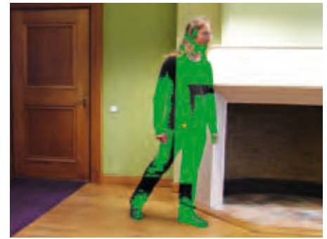
Figure 5. Here the detected pixels have been melded with the original image. The red spot marks the centre of mass of the detected motion.
