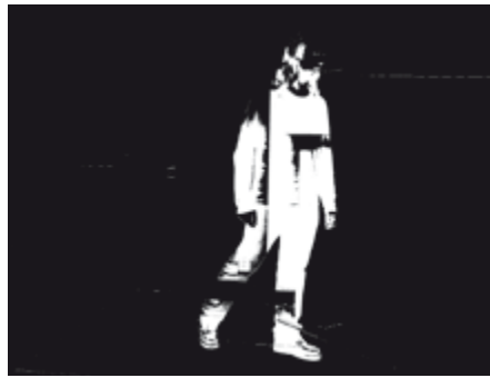
Figure 4. The result of the next step: the pixels in this image are white where the grayscale difference is greater than a defined threshold.
