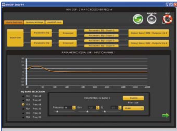
Figure 6. Every parametric equaliser of the two-way plug-in allows a maximum of six corrections (frequency, value, Q factor). Here a simple bass-boost has been realized.
