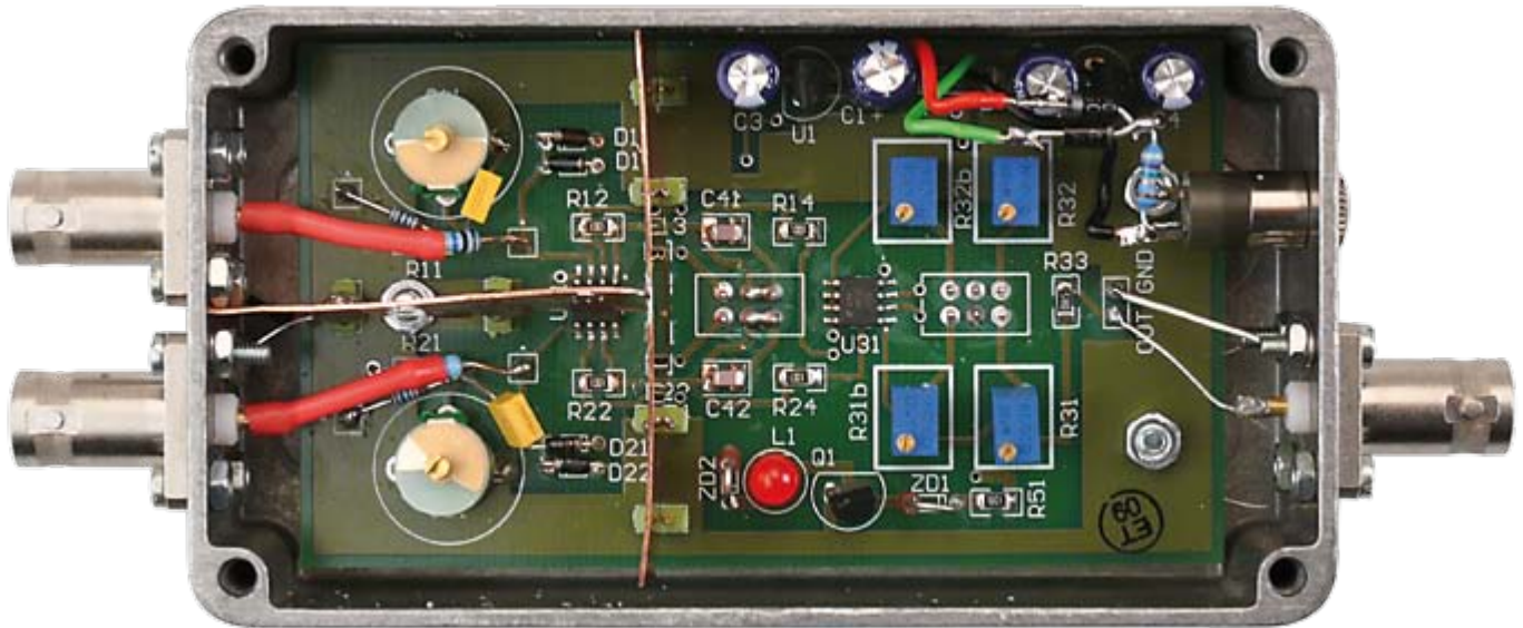
Figure 6. Completed circuitry with the printed circuit board inside the diecast aluminium box.
