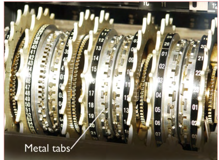
Figure 1. The coding wheels in a Lorenz machine were a wonder of precision metalworking.
