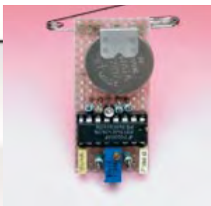
Figure 2. Fit the components as close together as possible on a piece of perforated circuit board to keep the finished circuit compact.
