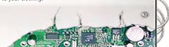
Figure 3. You can make an on/off switch from a safety pin, which also serves to pin the brooch to your clothing.
