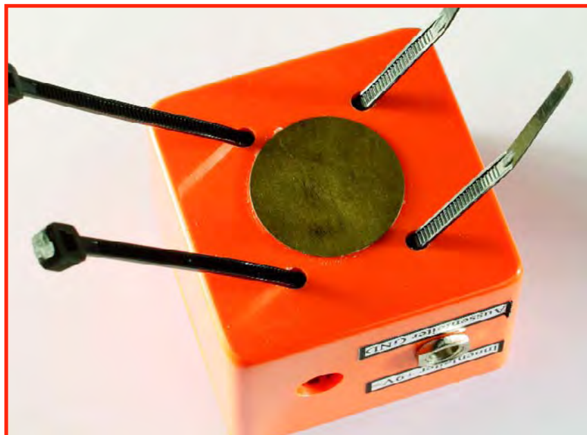
Figure 2. Two cable ties clamp the enclosure and sensor (glued onto it) to the hot water pipe.
