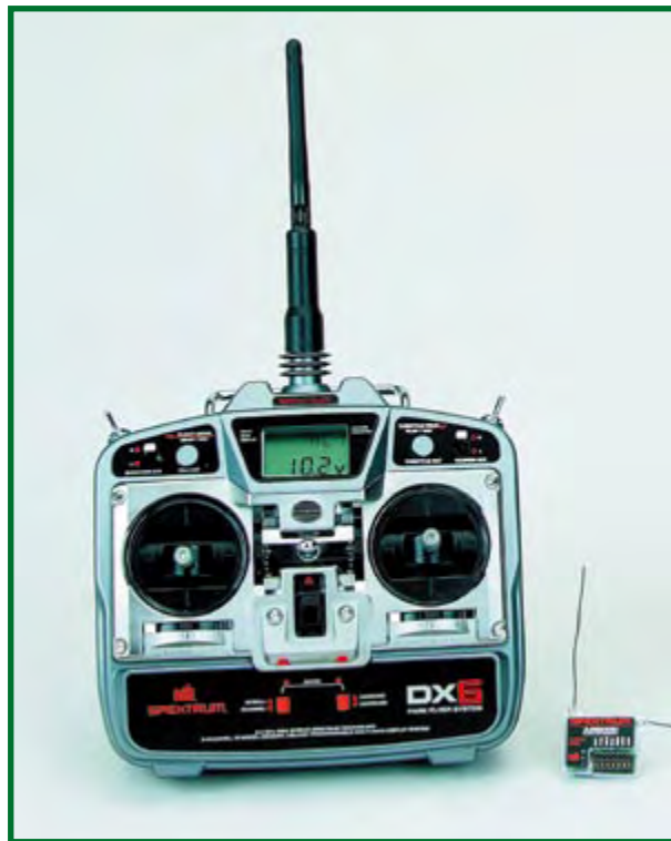
Figure 2. DX6 2.4 GHz model aircraft transmitter with receivers for six servo functions (Source: Graupner [6]).
