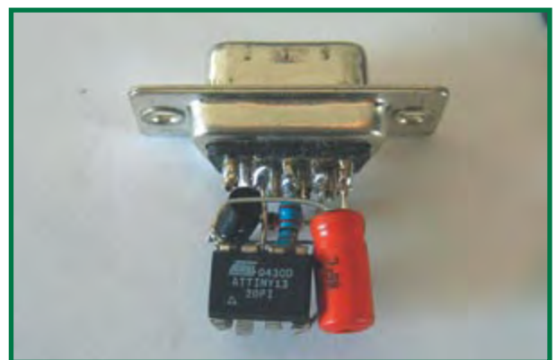
In this case a PCB would take up valuable space. Besides, it's much more fun to construct it like this.
