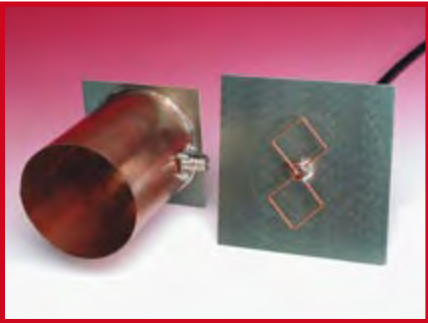
Figure 4. Prototype antenna and biquad antenna constructed in the Elektor Electronics laboratory.
