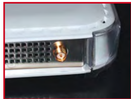
Figure 1. SMA connector on the rear panel of an access point.
