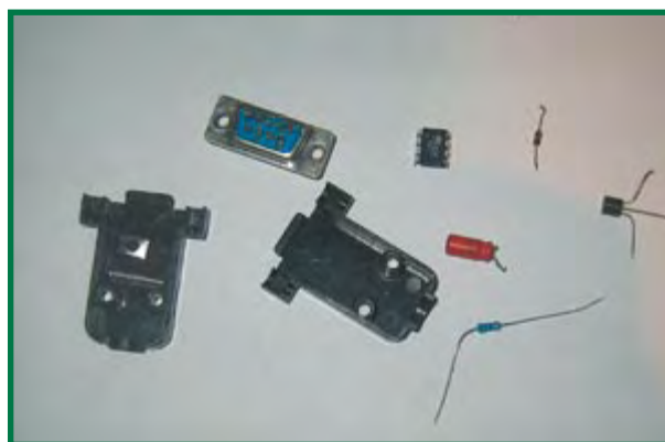
You only need five electronic parts, one DB9 connector & cover and some cable to build this project.
