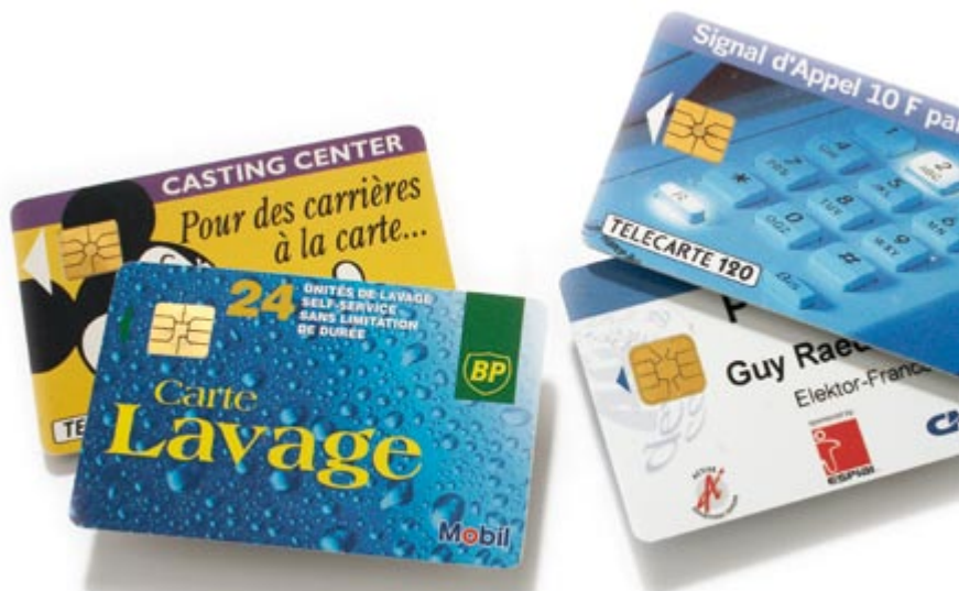
Old chipcards (left) still used the AFNOR standard, but these days they conform to the ISO standard (right), which is an international standard.
