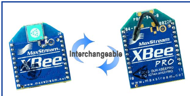
Figure 1. MaxStream uses a special logo to emphasise the interchangeability of the modules.
