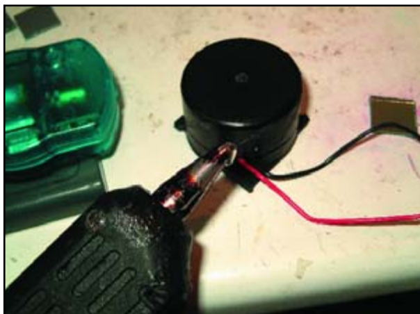
Hot glue is perfect to attach the little mirrors with varying angles.
