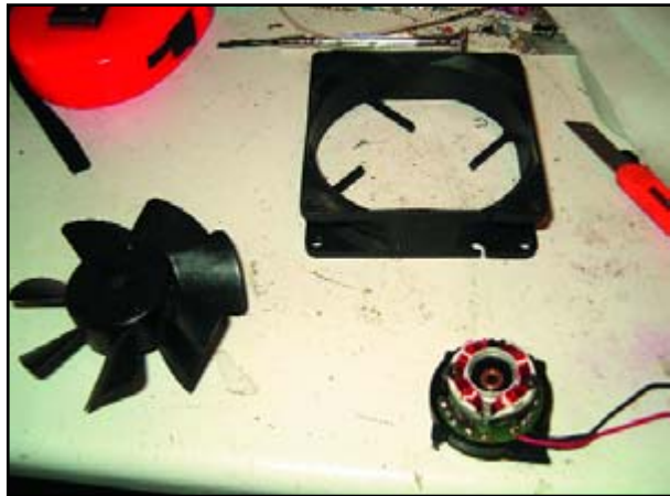
The frame we don't need for this project... ...just like the fan blades. In this way we are left with a nice, round 'puck'.
