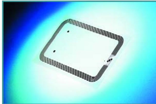
Figure 1. RFID label with antenna and chip.
