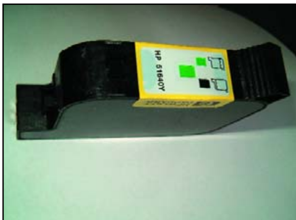
The cartridge concerned, the 51640M from HP, otherwise known as 'type-40'. According to sources on the Internet this cartridge can be refilled at least 10 times.
