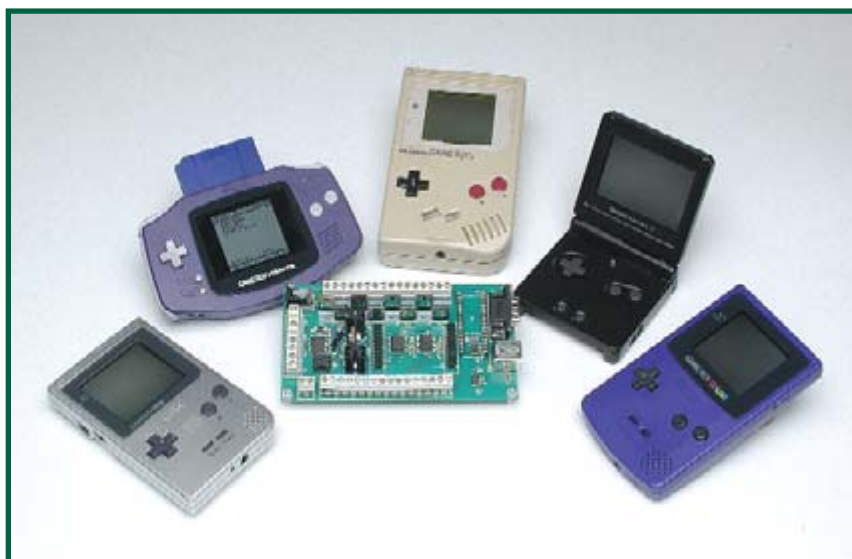
Figure 1. Suitable GameBoy models. The unit in the centre is the GBPLC I2C I/O Box, which drives the GameBoy fitted with a GBPLC module.
