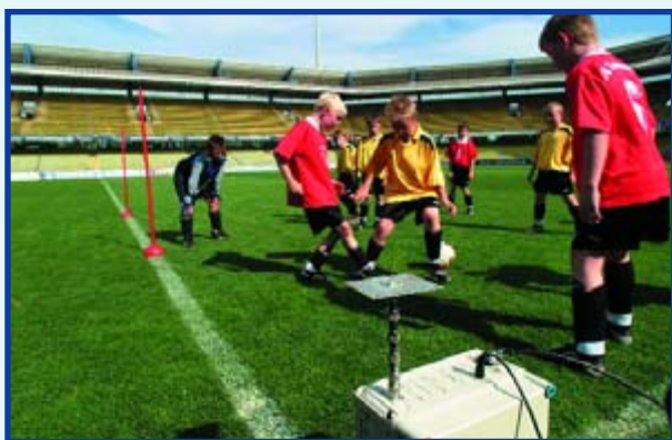
Aerials around the pitch perimeter detect time differences in the signal received from the smart ball which allows its position to be calculated (picture: Fraunhofer IIS).
