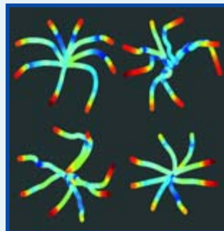
Traces recorded from the scalps of four individuals using the BCI system to move a cursor from the centre of a computer screen to targets around the edge. The cursor paths are shown, with colour representing speed at each point, from slowest (blue) to fastest (red).
