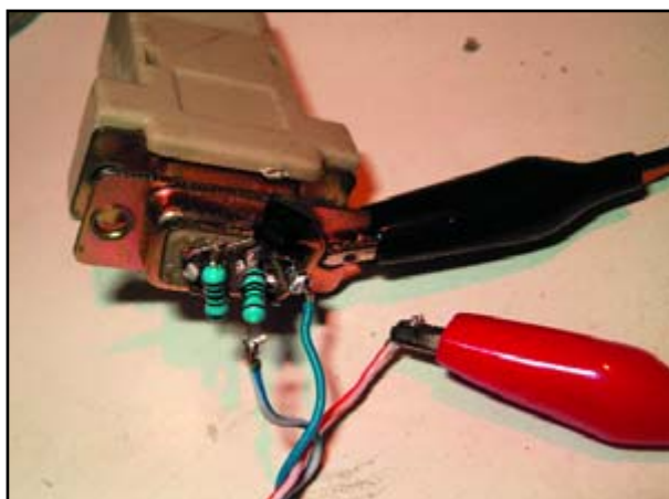
Since this circuit is only temporary (Fig. 1) it is built straight onto the DB9 plug without using a circuit board.
