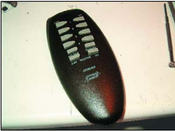
The transmitter. This is used to control the four outputs and the dimmer function. There is also a master switch that can turn all outputs on or off at the same time.
