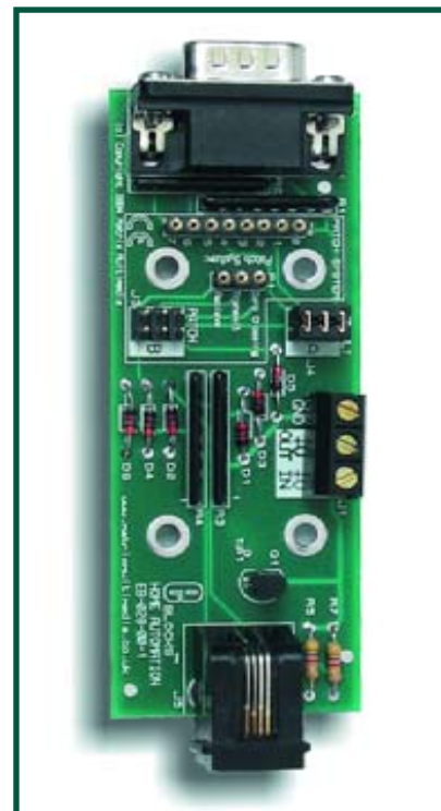
Figure 5. The E-blocks X-10 interface.
