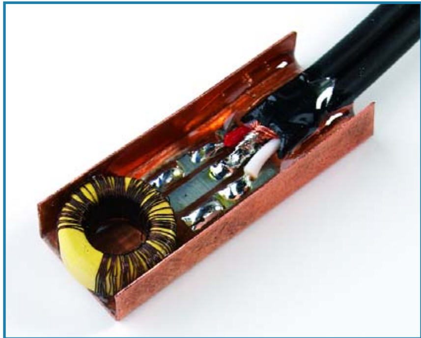
Figure 3. This is one way to implement the sensor. The copper enclosure provides sufficient shielding from interfering sources.
