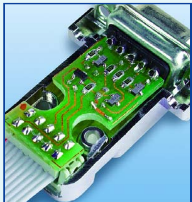
Figure 3. The circuit board with the SMD components fitted.
