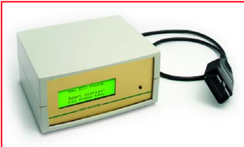
Figure 2. Prototype of the stand-alone OBD analyser.
