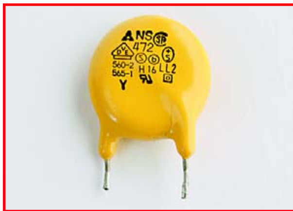
Figure 11. An approved Y-class capacitor.
