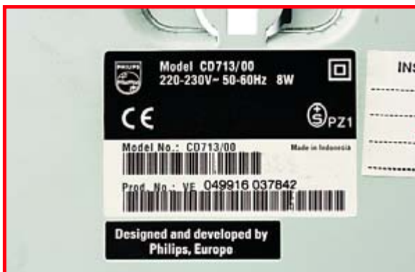
Figure 2. The symbol indicates a Class II device.
