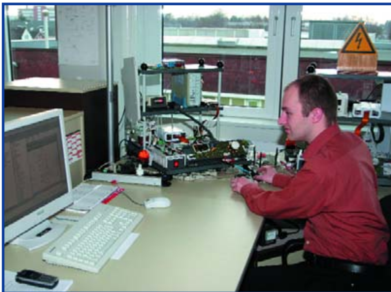
Figure 4. Andreas Lux seen here testing software modules in an emulator environment. Water levels in the machine are simulated with the help of a pressure pump.
