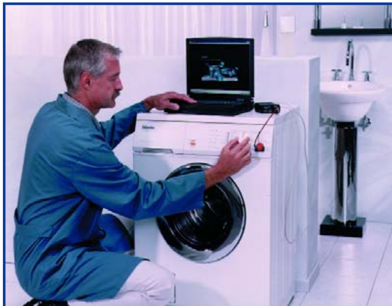
Figure 1. The washing programme parameters can be altered via an optical service interface (covered here by the suction cup). This allows the machine wash cycle to be matched to the requirements of any future (more efficient) washing powder.
