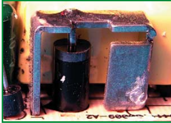
Figure 10. Diode with thermally and electrically conducting heatsink.
