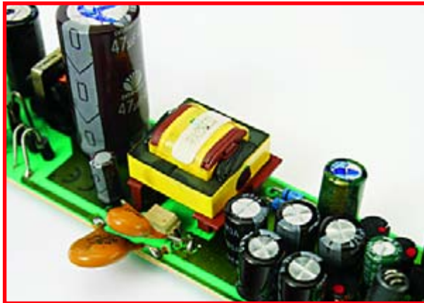
Figure 5. Mounted transformer, optocoupler and Y-class capacitors.
