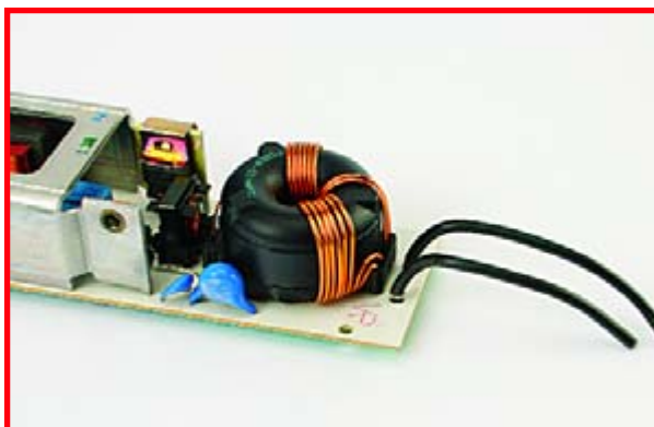
Figure 3. Toroidal transformer in a supply for a halogen lamp.
