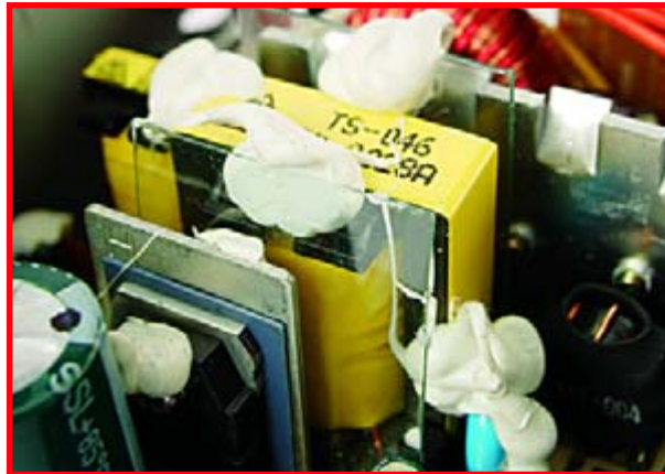
Figure 10. Insulating sheets are fitted between the transformer and the heatsinks.
