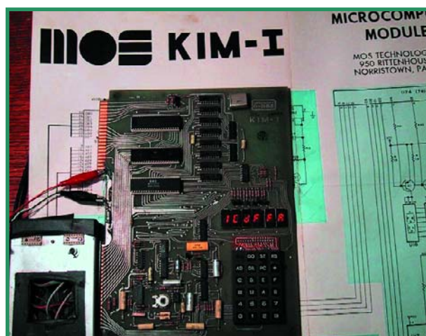
Figure 1. The KIM-1 computer, developed by MOS Technology. Input was via a hexadecimal keyboard, for the output a 6-digit LED display was present.
