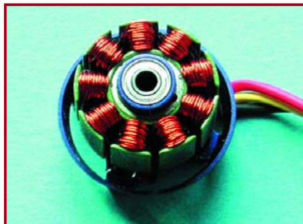
Figure 2. A high fill factor is important: here there is some room for improvement!
