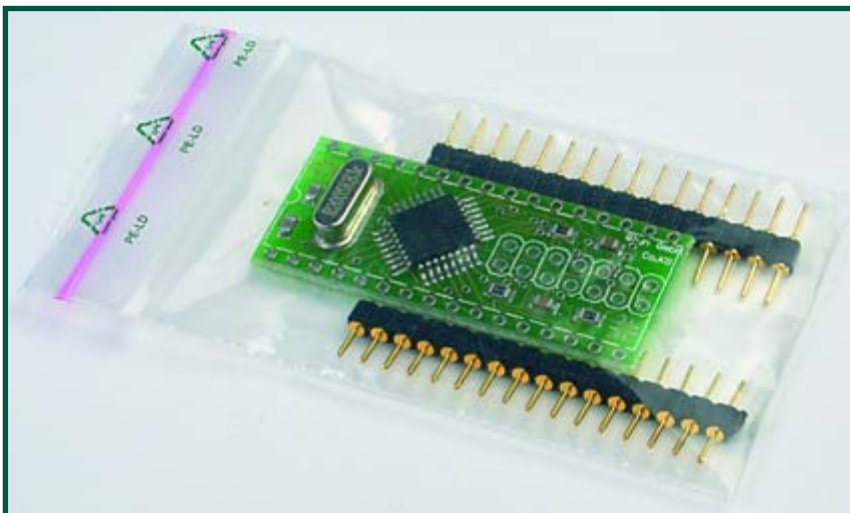
Figure 1. The hardware you can order from us at low cost forms a complete microcontroller system.
