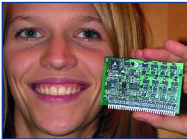
Figure 4. This piezoelectric motor driver kit from Trinamic offers four output signal channels. (Source: Trinamic).
