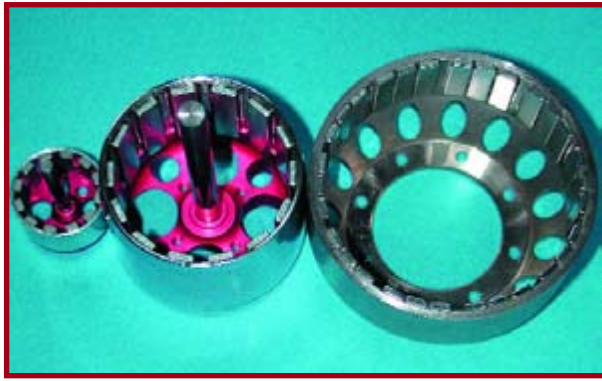
Figure 12. The distance between the magnets in a multi-pole machine (in this case with exterior rotor) should not be too small. Right, a ten-pole rotor where one pole is formed by each group of three adjacent magnetic strips.
