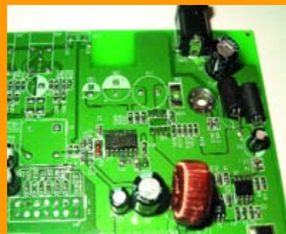
Close-up of the 5 V supply (still to be built). This is required for the USB port. The empty space suggests that the voltage would be regulated by U10 and a handful of passive components...
