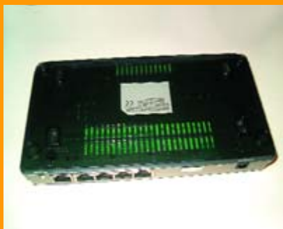
There are five Ethernet ports, one power connector and a reset button, but no USB socket... and we do need one of these. We have to do something about that.
