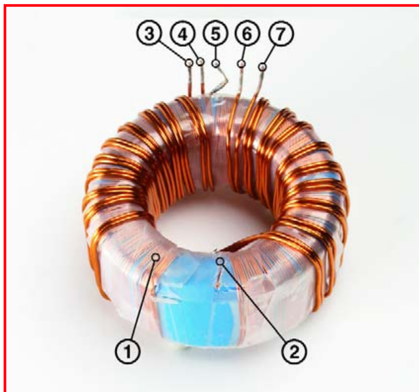
Figure 8. This shows how you should wind the transformer. Although this is version 2.0 of the transformer (as opposed to version 3.0 in the photo of the prototype), the winding method is the same. Legend: ① = C4 in the schematic; ② = C1; ③ = B2; ④ = A2; ⑤ = C2 and C3; ⑥ = B1; ⑦ = A1.
