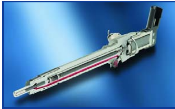
Figure 2. A piezoelectric valve in a diesel injection pump. The grey piezo actuator at the right moves the needle in the nozzle. (Source: Siemens VDO)
