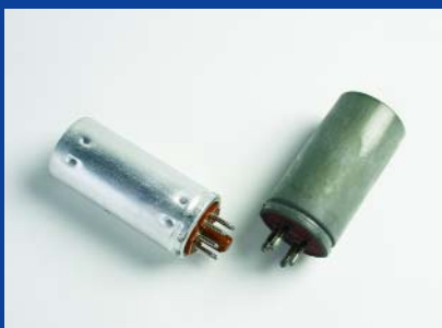
Vibrators for portable or semi-mobile valved equipment are often dead or worn out. Even new ones may not 'start' owing to internal contact oxidation. Be sure to know the voltage and base pinout.
