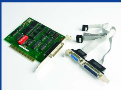
Contrary to popular belief, PC junk has little to offer in the way of useful parts. This serial I/O board might be persuaded to give up its 18.432MHz UART xtal, DIP switch and sub-D connectors.
