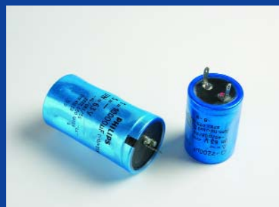
These large electrolytics rated for 63 V are NOS and may look great for your restoration work on a 1980's PSU but be warned — their ESR was found to be poor due to dried out electrolyte inside.
