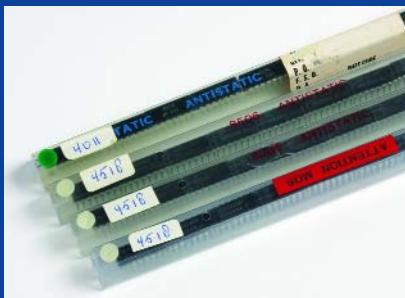
CMOS ICs in static protective tubes. Be careful, the type labels are handwritten so the devices are not genuine surplus from a distributor, test house or manufacturer. That's not to decry the value, though.
