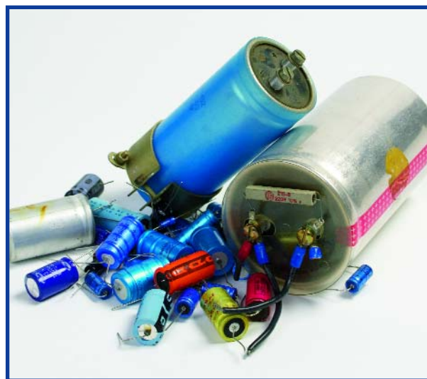
Figure 3. Electrolytic capacitors are a problem for waste disposal. Older types can contain harmful substances such as PCBs.
