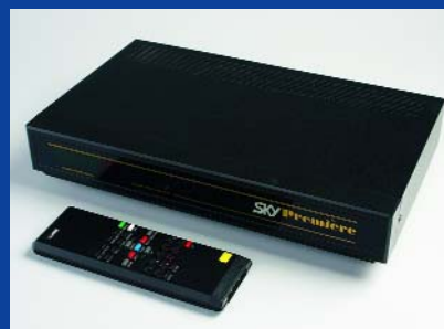
Intact equipment of the NIB variety! Watch 23cm amateur television (ATV) or Hotbird channels using this analogue satellite-TV receiver. But then, at a fiver you get a nice display, remote control, switch-mode PSU and a bunch of connectors.
