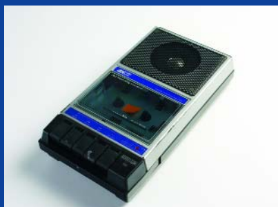
At just one pound, this discarded cassette recorder was good value for its 6 V DC motor, electret microphone, audio playback amp, loudspeaker and a few PCB mount jack sockets.
