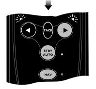
Fig 3.4 - Initiating Port Autotack in Sail To Wind Mode
