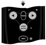
Fig 4.3 - Entering Calibration Mode
