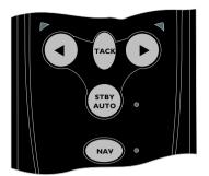
Fig 2.1 - Tillerpilot keypad
