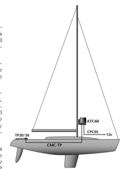
Fig 3.5 - Using TP20 / TP30 with external compass
