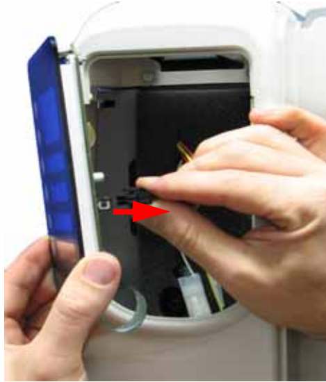
Figure 4-25: Disconnecting the J1 connector
