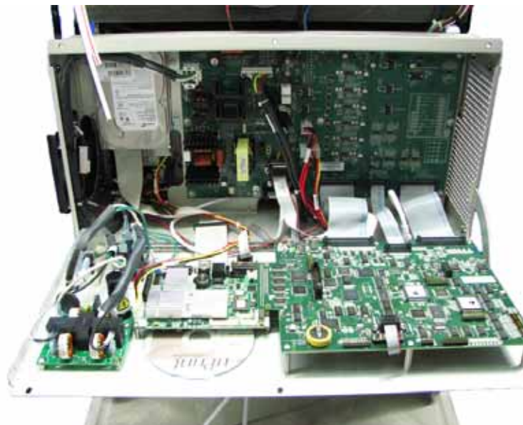
Figure 4-34: Electronics bay with cover lowered
