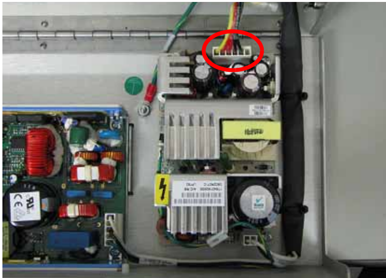
Figure 4-86: SK2 connector location
