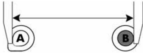
Figure 5-335: Measuring distance from outside edges of A and B
