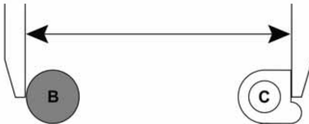
Figure 5-285: Measuring distance from outside edges of B and C
