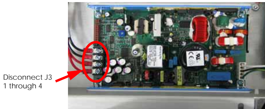
Figure 4-80: J3 1 through 4 connector locations
