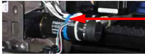
Figure 4-106: Wire tie location
