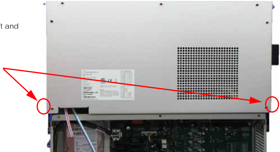
Figure 4-36: Upper electronics bay cover bottom mounting screw locations
