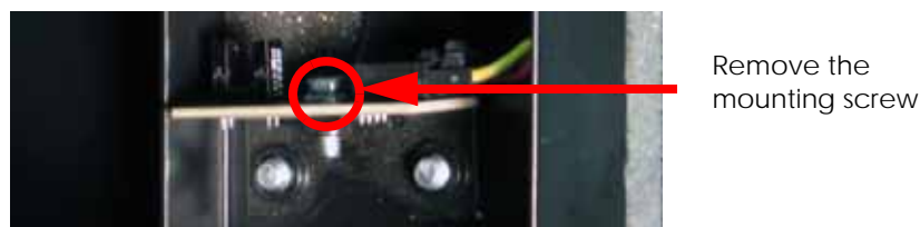
Figure 4-155: Y home sensor mounting screw location
