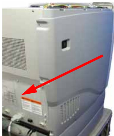
Figure 4-20: Removing the left side panel
