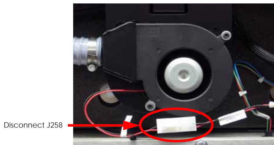
Figure 4-92: J258 cable location
