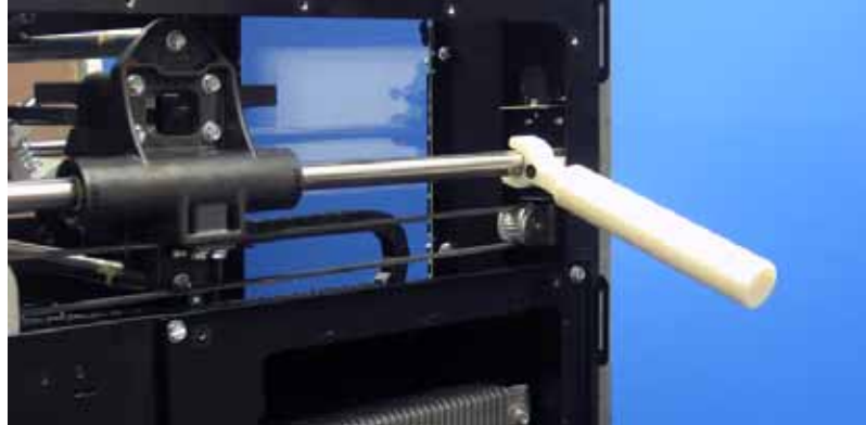
Figure 4-232: XY guide rod leveling fixture
