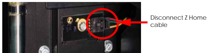
Figure 4-238: Z home sensor cable location
