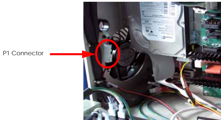
Figure 4-40: Electronics bay cooling fan connector location
