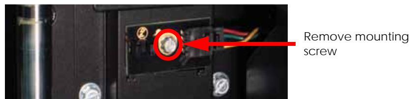
Figure 4-239: Z home sensor mounting screw location
