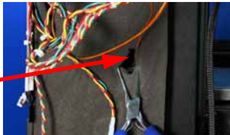
Figure 4-258: Strain relief clip location
