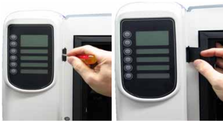
Figure 4-23: Opening the display panel access hatch
