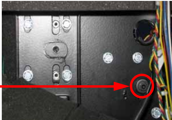
Figure 4-218: Left side rear Y guide rod mounting screw location
