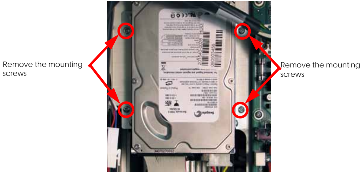
Figure 4-65: Hard drive mounting screw locations
