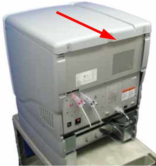
Figure 4-18: Top panel removal
