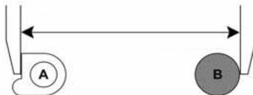
Figure 5-299: Measuring distance from outside edges of A and B
