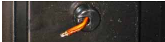
Figure 4-259: Bending the thermocouple
