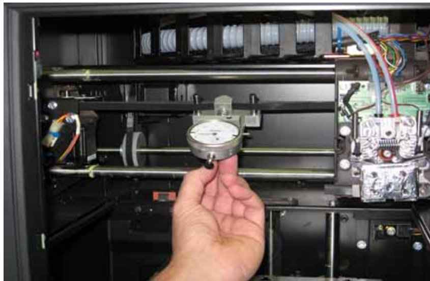
Figure 4-168: X belt tension location
