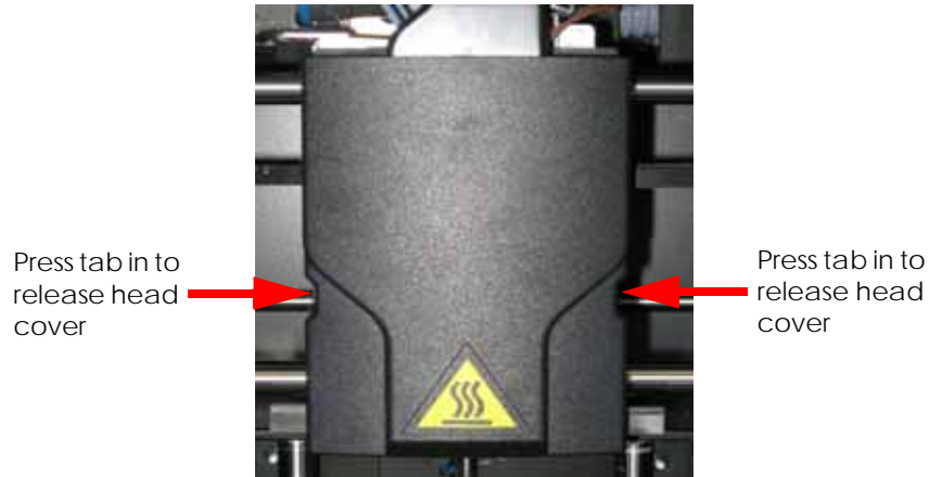
Figure 4-127: Head cover tab locations
