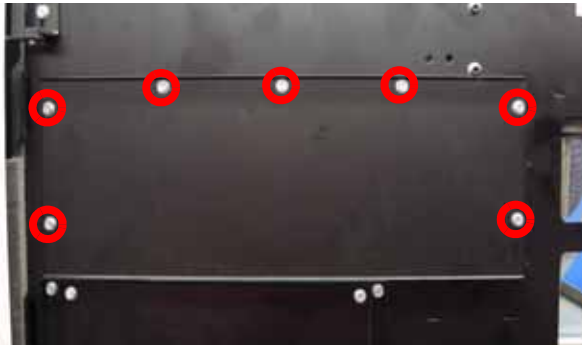
Figure 4-114: Right side access panel mounting screw locations
