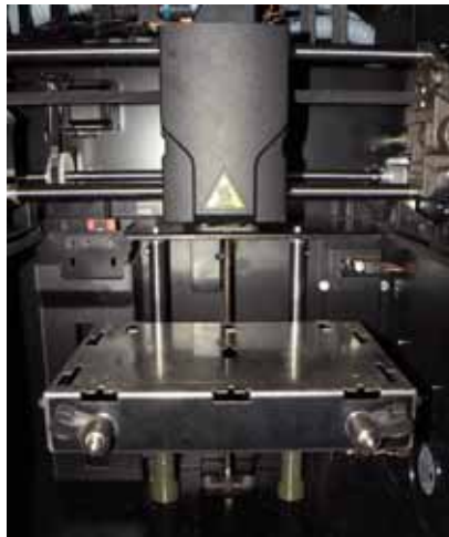
Figure 4-273: Marking the 4 corners of the Z stage
