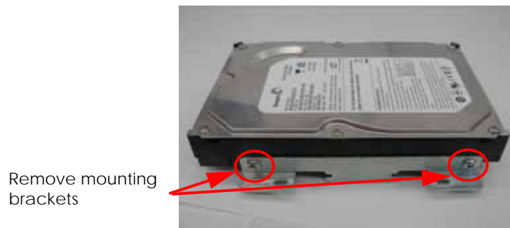
Figure 4-62: Hard drive mounting bracket screw locations
