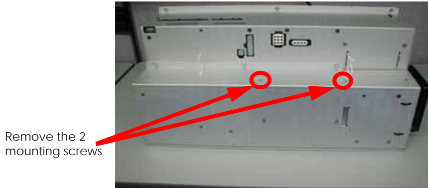
Figure 4-82: Removing the 2 mounting screws from the top of the panel
