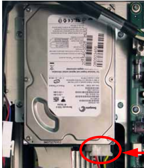
Figure 4-63: Hard drive power cable location
