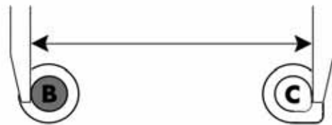
Figure 5-317: Measuring distance from outside edges of B and C
