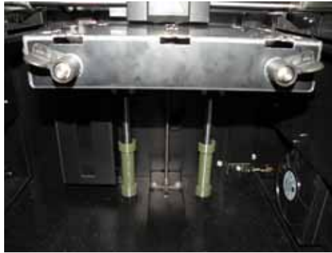
Figure 4-227: Z guide rod stand off locations
