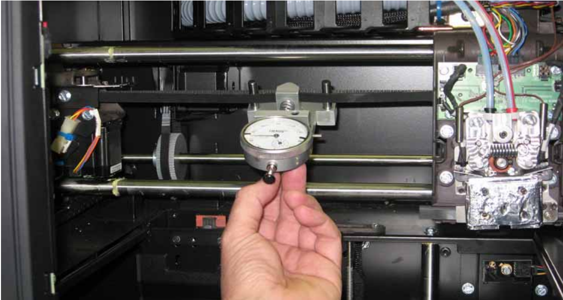
Figure 5-354: X belt tension location
