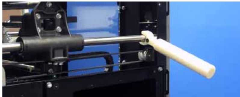
Figure 5-363: Y guide rod adjustment location
