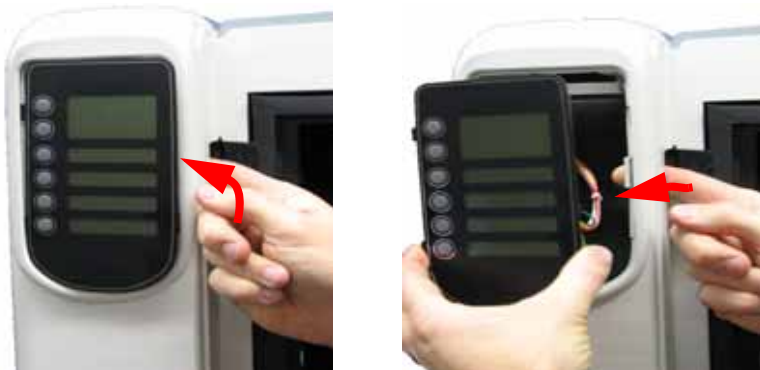
Figure 4-24: Removing the display
