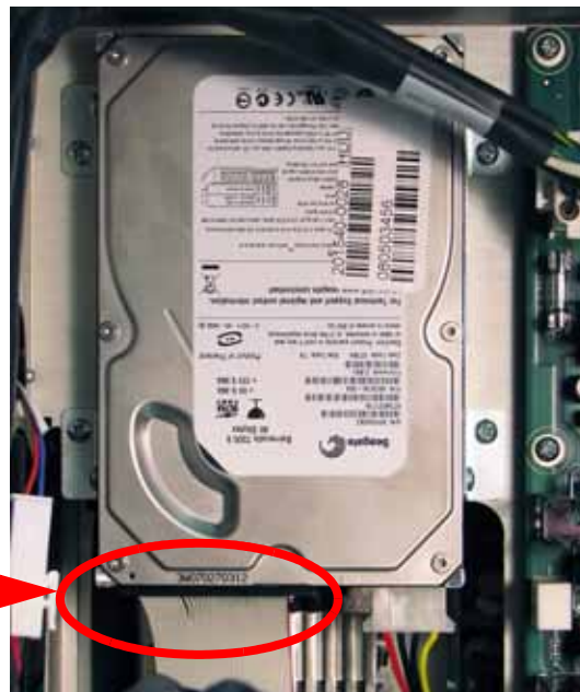
Figure 4-64: IDE cable location
