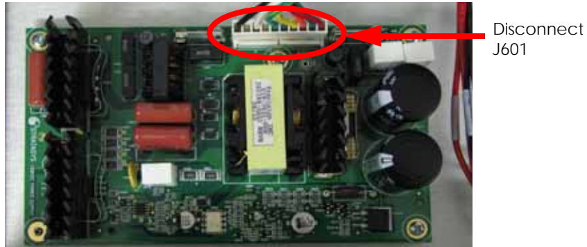
Figure 4-90: J601 connector location
