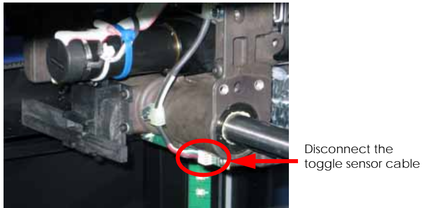
Figure 4-101: Toggle sensor location
