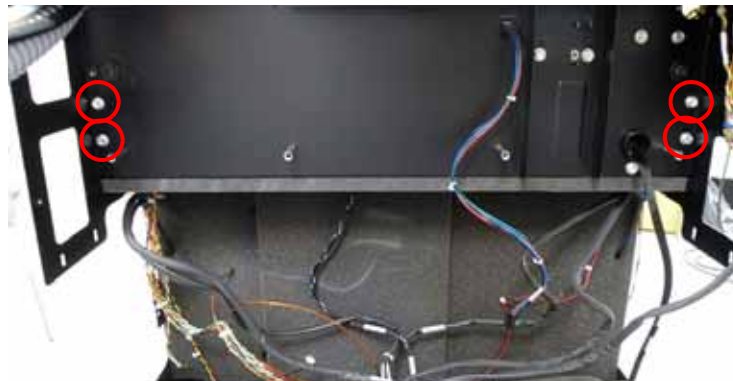
Figure 4-201: Upper Y drive rod mounting screw locations
