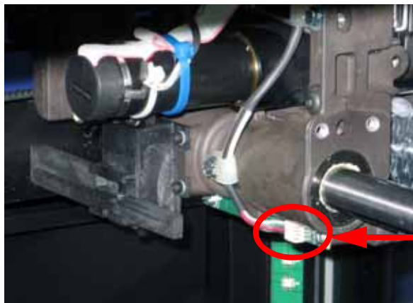
Figure 4-134: Disconnect the toggle sensor cable from the toggle sensor
