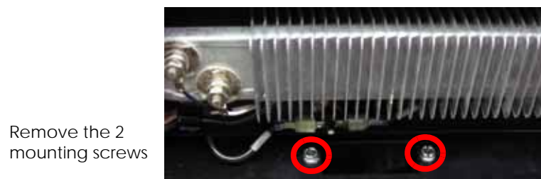
Figure 4-245: Left side chamber fan mounting screw locations
