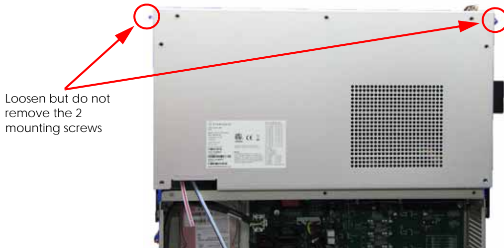
Figure 4-35: Upper electronics bay cover top mounting screw locations
