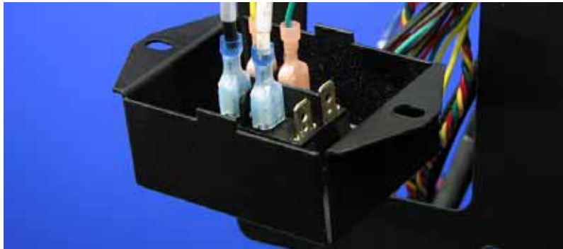
Figure 4-76: Power switch connector locations
