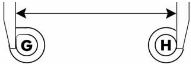
Figure 5-324: Measuring distances from outside edges of G and H
