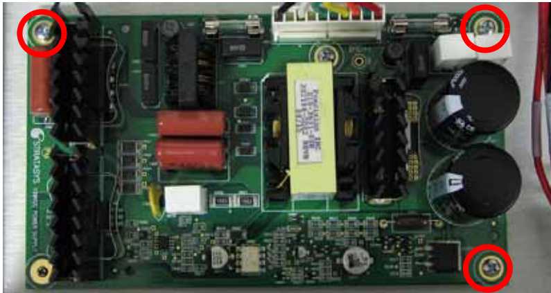
Figure 4-91: 120 VDC mounting screw locations
