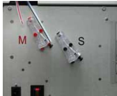
Figure 4-32: Removing the filament tubes from the Y connectors
