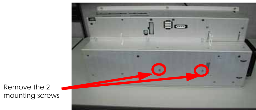
Figure 4-81: Closing the rear panel of the electronics bay
