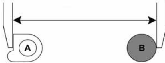
Figure 5-284: Measuring distance from outside edges of A and B
