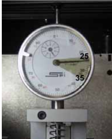
Figure 4-169: Gauge reading at correct X belt tension (Shading indicates acceptable range)
