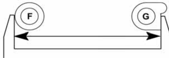
Figure 5-302: Measuring distances from outside edges of F and G
