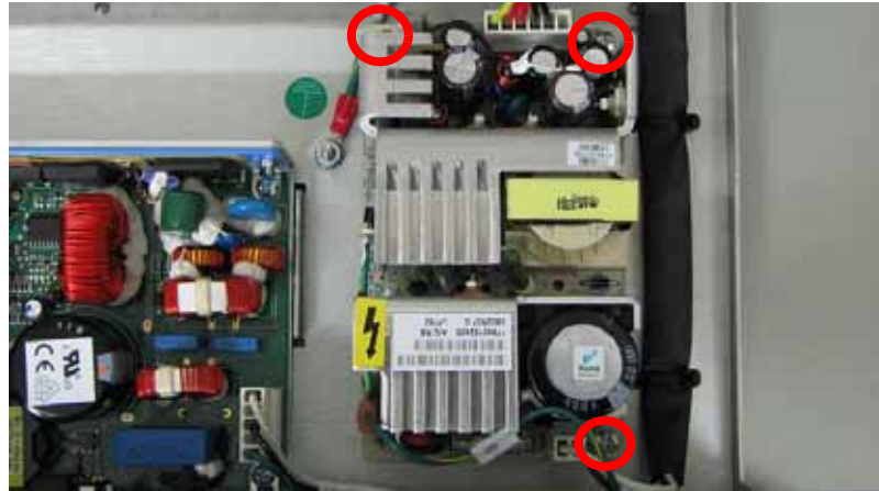
Figure 4-88: 5/12 VDC supply mounting screw locations
