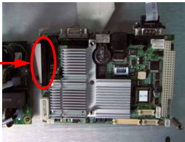
Figure 4-49: SBC IDE ribbon cable location
