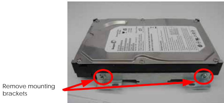
Figure 4-66: Hard drive mounting bracket screw locations
