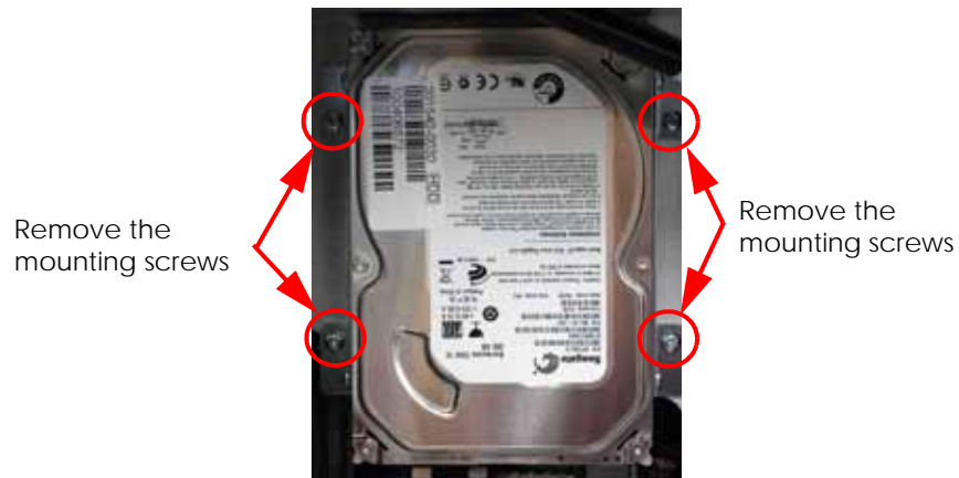
Figure 4-61: Hard drive mounting screw locations
