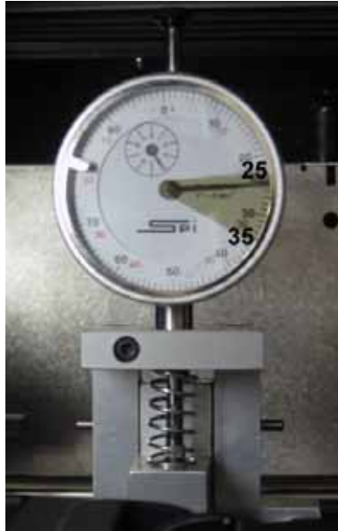
Figure 4-235: Gauge reading at correct X belt tension (Shading indicates acceptable range)
