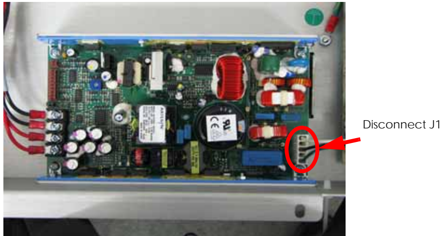
Figure 4-79: J1 cable location
