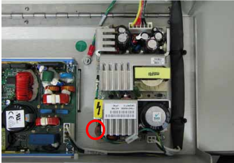
Figure 4-85: J2 spade connector location
