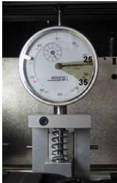
Figure 5-355: Gauge reading at correct X belt tension (Shading indicates acceptable range)
