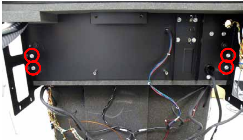
Figure 4-187: Upper Y drive rod mounting screw locations
