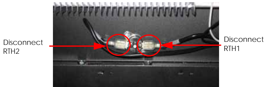
Figure 4-253: RTH1 and RTH2 spade connector locations
