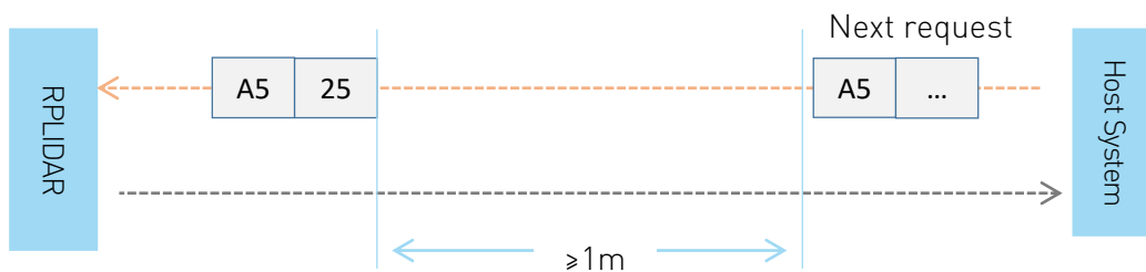
Figure 4-2 The Timing Sequence of a STOP Request
