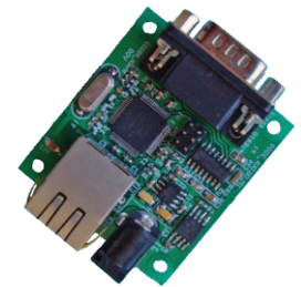
RS232 Gateway to Ethernet (Part # TIPL402 )
