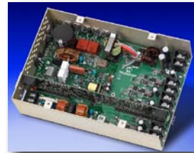
The free, downloadable Microchip ac/dc reference design has one four-layer board for digital signals and another for the other power stages
