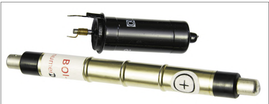
Figure 2: Two examples of common metal-wall Geiger-Müller tubes.
