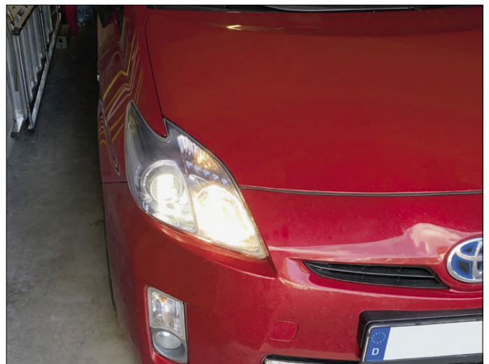
Figure 10: Tadaaa! My Prius with DIY-tuned low beam. You can see the slightly less yellowish colour of the low beam, which is now run at 13.4 V (high beam at only 11.8 V).
