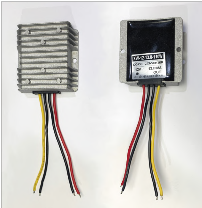
Figure 7: DC/DC converter: 9–14 V in and 13.8 V out, weatherproof, and encapsulated in a sturdy aluminium casing.
