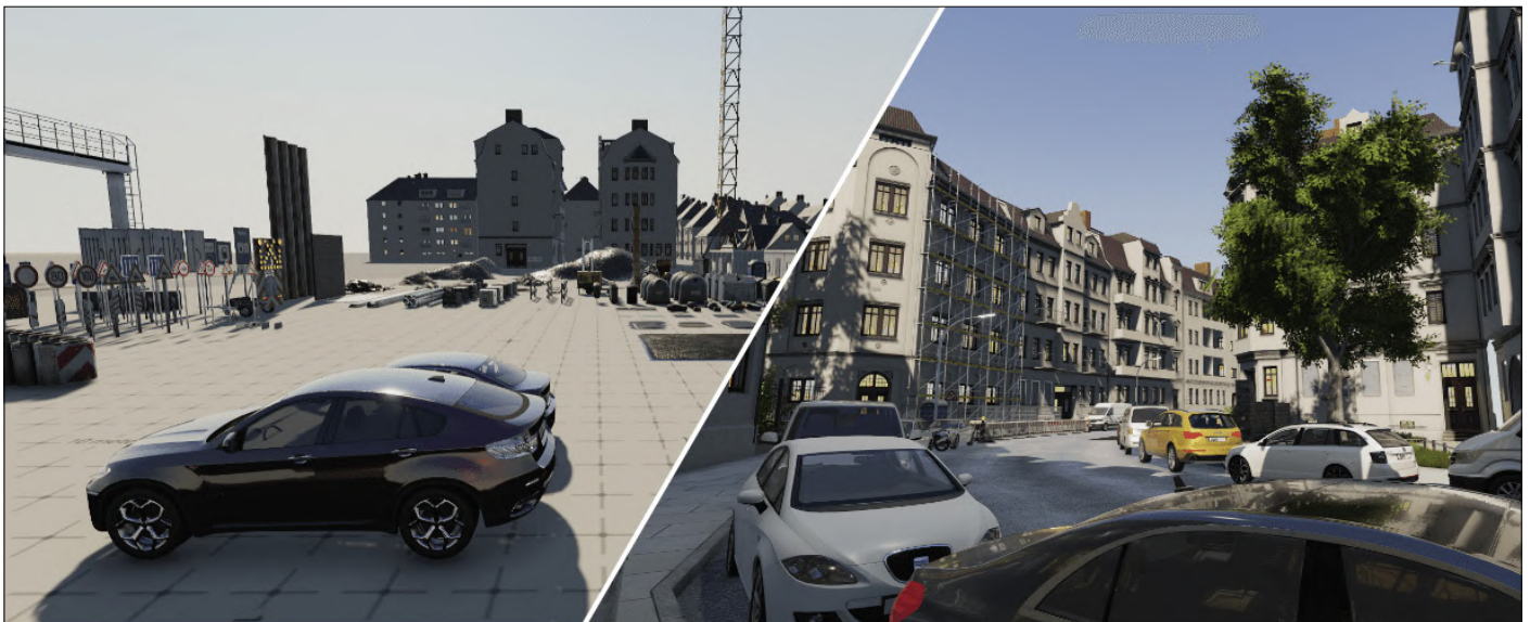
Figure 8: Simulation systems based on 3D engines are common in AV - here an example of AAI with some basic building blocks such as road signs or a construction site on the left side (virtual image: AAI).
