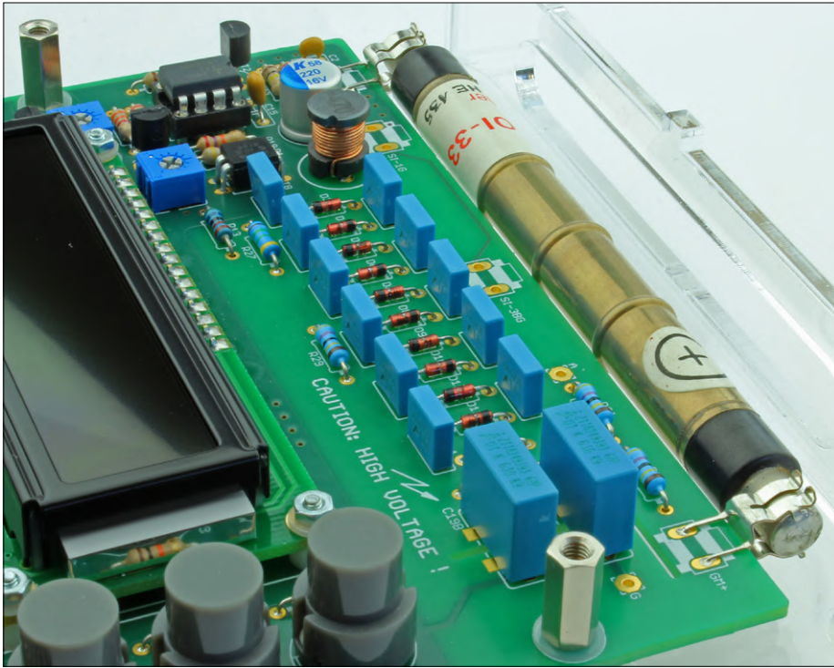
Figure 5: The high-voltage supply powers the Geiger-Müller tube.
