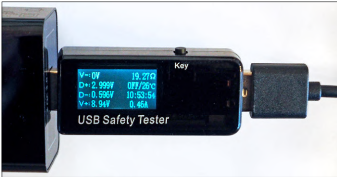
Figure 8. The Yootech Qi pad switches into 5-W mode taking 9 V.
