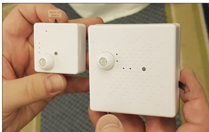
Figure 2. Two identical multi-sensors side by side: one using LoRa and the other for NB-IoT data radio ( www.tektelic.com ).
