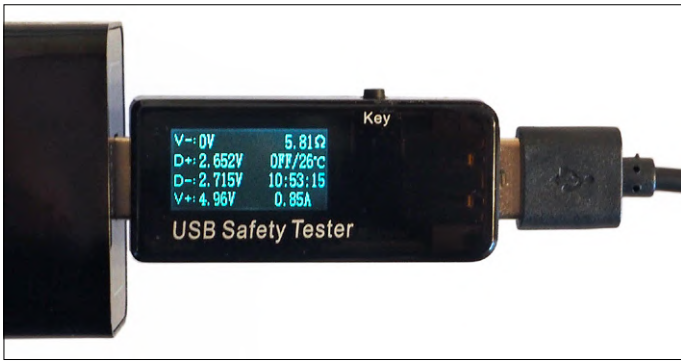
Figure 7. The 5-watt Qi charging pad from Pulesen draws 0.85 A at 5 V.
