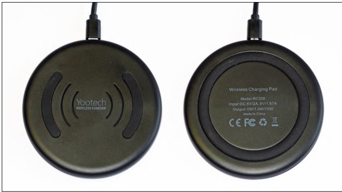
Figure 3. One smooth puck: The Yotech 10 W RC200 Qi charging pad.
