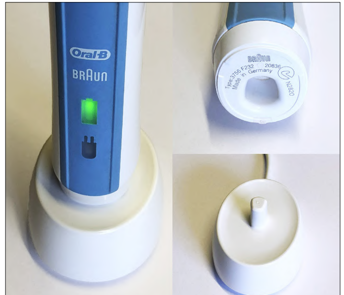
Figure 1. The forerunner to Qi: inductive toothbrush charging by Oral-B.
