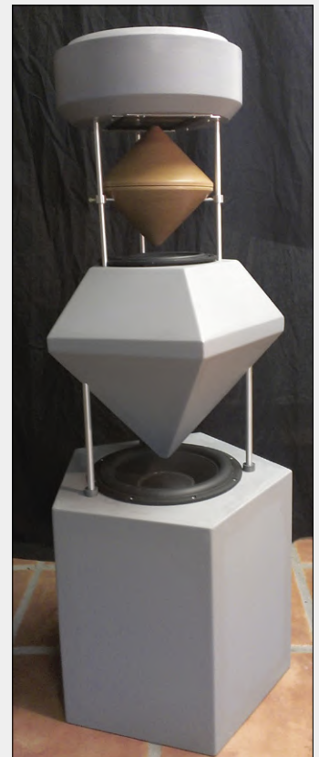
Figure 8: The three-way loudspeaker system as built by the author, based on the considerations in this article.
