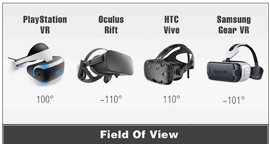
Figure 3: FOV comparison of VR headset displays. Source: VRGlassesHeadsets.com. Source: [2]
