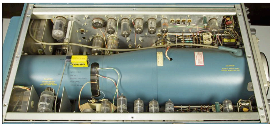
Figure 3. Inside top view of the Tek 556 and its massive dual-beam (not: dual-trace) CRT. It's a good thing we now have LCD and LED screens on our 'scopes.
