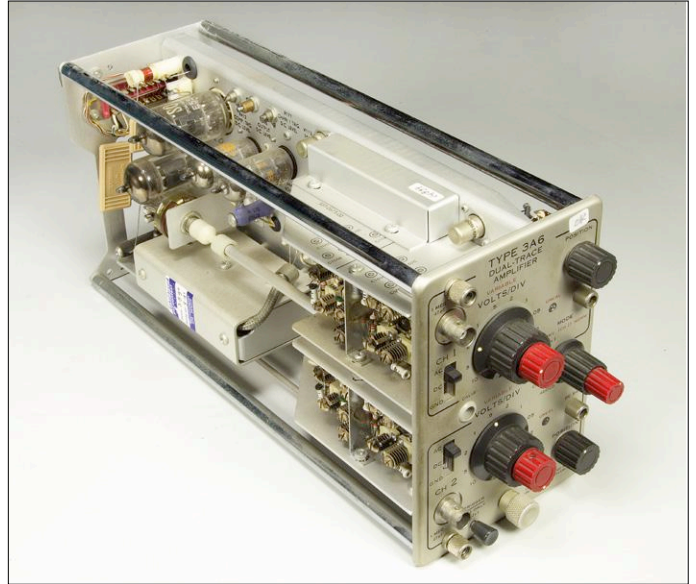
Figure 5. Tektronix 3A6 dual-trace plug-in. Two of these in a 556 'scope give you four crisp traces from two electron beams.
