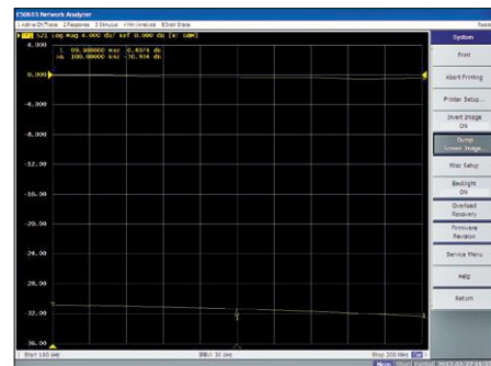
Figure 7. Screenshot showing the frequency response at minimum (0 dB) and maximum (31 dB) attenuation.
