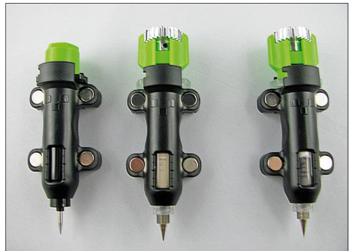
Figure 3. Tool modules of the Voltera V-One.
