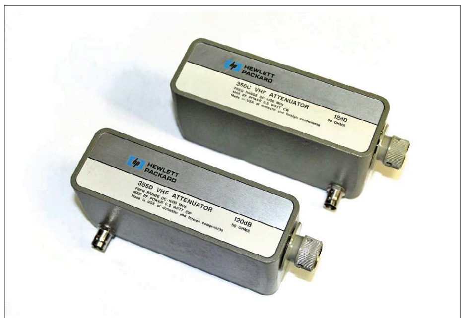
Figure 1. Example of a VHF attenuator by HP, long since out of production.
