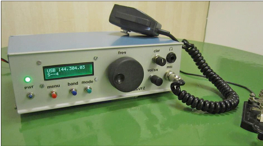
Figure 8. The prototype built by the author doing USB at 144 MHz.
