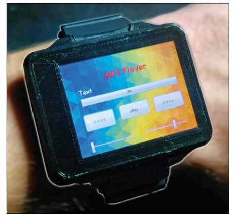
Figure 4. Thanks to a dedicated decoder IC the nWatch can be used as MP3 player.
