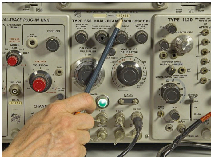
Figure 1. Central area on the Tektronix 556 oscilloscope front with controls and connectors common to both beams.
