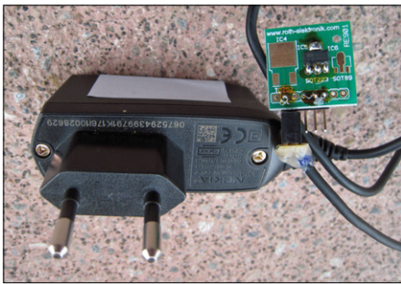
Figure 3. Together with a mains adapter Miroslav (using the circuit in Figure 2) built his first Li-Ion charger. The only drawback? You can't see what's happening.
