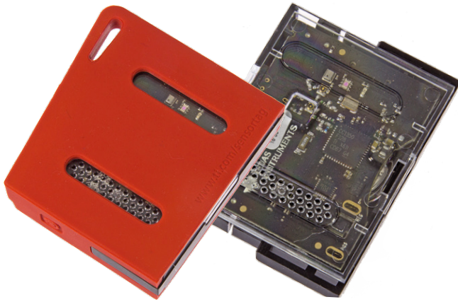
Figure 10. The CC1350 SensorTag lurks inside its enclosure.
