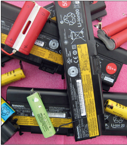
Figure 1. A bundle of rejected laptop batteries. Many of the cells are too good to just chuck out.
