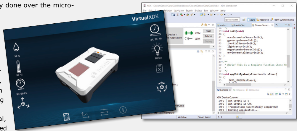
Figure 7. On the left, the main view presented by the VirtualXDK app. On the right, the Eclipse-based XDK Workbench holds few surprises: only the programming procedure and use of the bootloader will be unfamiliar, but learning these will not present much of an obstacle to the experienced developer.
