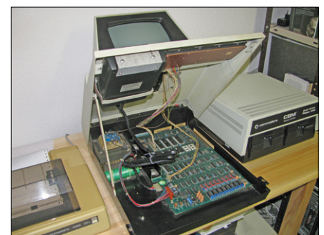
Figure 4. The case can be released by undoing just two screws.
