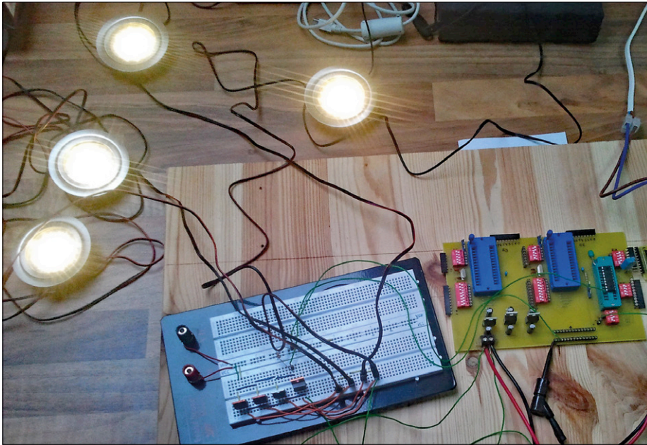
Figure 1. Rapid prototype construction by the author: programmer with microcontroller and four MOSFETs on a breadboard.
