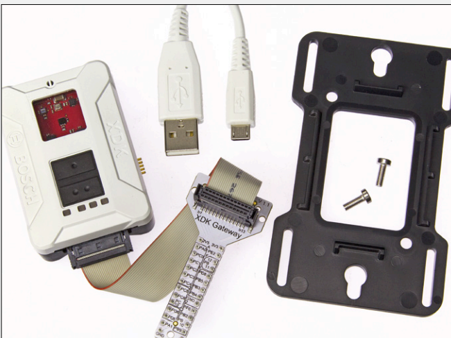
Figure 6. The main components of the XDK110 kit: even a wall fixing bracket is included. The photo shows how astonishingly small the device is.
