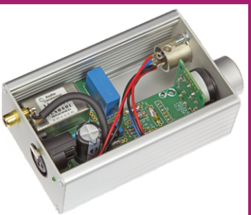
Microphone Preamp with professional specs
