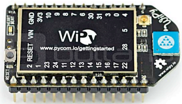
Figure 4. The WiPy is similar to the ESP8266-based NodeMCU board, but with a CC3200 ARM Cortex M4 instead.
