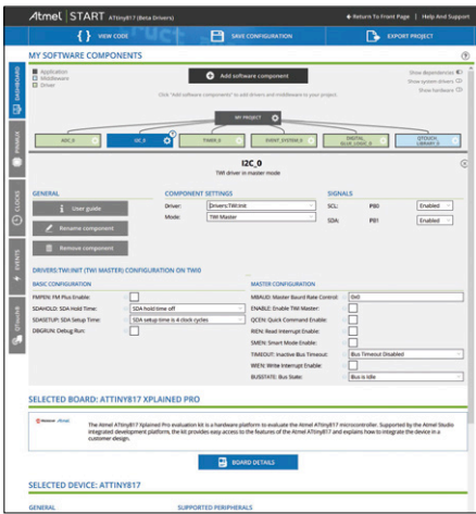
Figure 6. A screenshot of the Atmel START online environment. Each of the elements listed towards the top of the screen can be configured in detail before importing the customized project into Atmel Studio 7.
