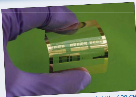
These tiny transistors with a bandwidth of 38 GHz were engraved and printed on a flexible substrate (photo courtesy of Jung-Hun Seo).
