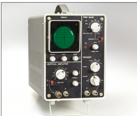
Figure 7. The BEM005 oscilloscope. Note again that this instrument was built from a kit of parts.
