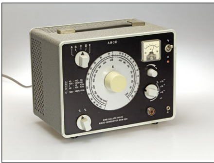
Figure 4. The BEM004 signal generator. Note that this is not a commercial instrument from MBLE but built from a kit of parts.
