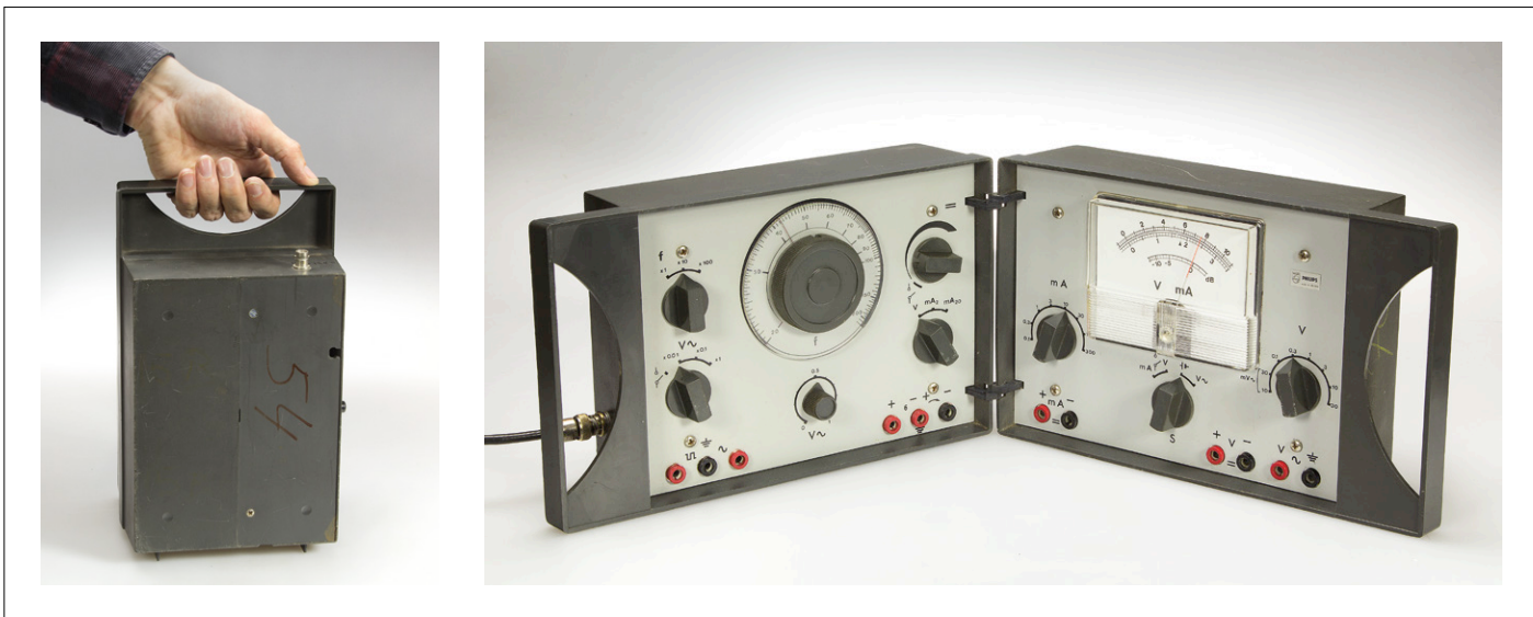
Figure 12. With a Belgian pinch of salt MBL's BEM045 multi-instrument can be called an electronics lab in a box. Note though that this was never a kit for home assembly but an important adjunct in Philips' PRACTRONICS course for audio and acoustic engineering.
