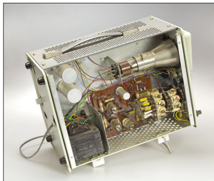
Figure 8. Inside, the BEM005 has plenty of space. Note the use of "printed wiring boards" (PWBs) in combination with vacuum tubes, which as we know is felicitous only if quality tube sockets are used in combination with proper soldering and solid copper traces.
