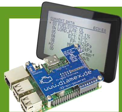
OBD2 Handheld with Raspberry Pi and new diagnose software
