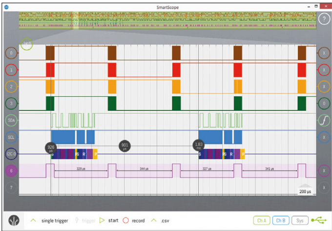
Figure 2. Interface to a 5-MP RGB image sensor. The bottom lines are the HSync and VSync, the top four lines contain actual pixel data. D4 and D5 are the Data and Clock lines of the I 2 C channel, with a decoder added to decode their data.
