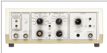
Figure 1. To kick off in ABS: Elektor Pulse Generator, mid 1980s. Sorry about the missing cap on the 0.1–1.0 Repetition Time variable control.
