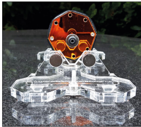
Figure 1. The magnets on the axle are suspended by magnets fixed in the frame.
