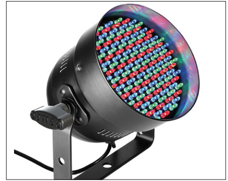
Figure 10. Cameo type CLP56RGB05PS PAR stage effect light with 151 colored LEDs and a power rating of around 30 W at 230 V. Not only does the light sport a DMX interface for remote control, it also has a built-in microphone to enable 'light organ' effects.
