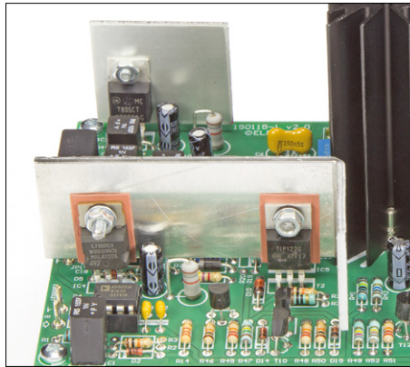
Figure 4. Two of the heatsinks are home-made from aluminum sheet metal with a thickness of 1 mm or 2 mm, respectively. The small one is for IC3, and the large one is for IC4, IC5 and T2.
