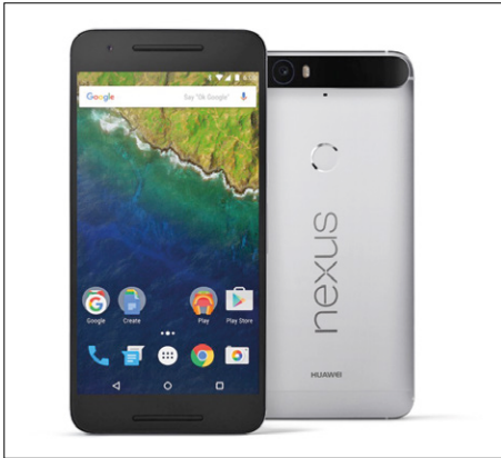
Figure 14. Google Nexus 6p: the OLED display on this reasonably-priced smartphone has a resolution of 2560x1440 pixels.
