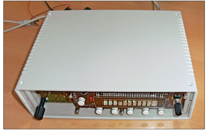
Figure 2. Lid on, firmware in: the kitchen Internet radio in operation. The electronics is visible through the acrylic front panel.
