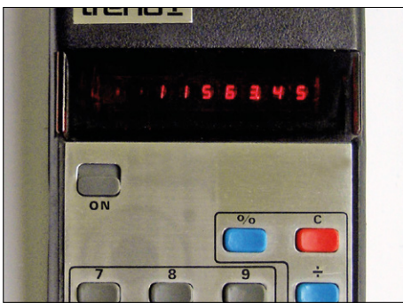
Figure 4. The first mass-market pocket calculators used tiny red seven-segment LED displays. (Source: Erhaka, Wikimedia Commons ).
