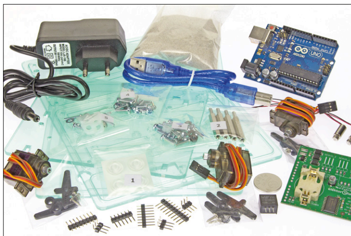
Figure 1. The kit contains all the parts (including the AC adapter) necessary to build the Sand Clock. However, you have to program the Arduino yourself using the free download software.
