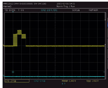
Figure 7. The roll parameter. The display shows an 'r' and no staircase, which means that a single recording will be displayed.
