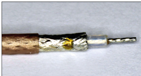
Figure 5. The PCB end of the coaxial cable looks like this when correctly stripped and tinned.
