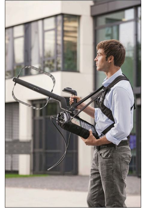
Figure 4. Mobile measuring receivers with directional antennas help operators monitor operational networks and identify interference.
