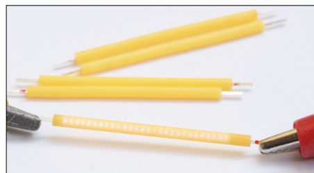
Figure 3. At very low current you can see the individual LEDs on the substrate.
