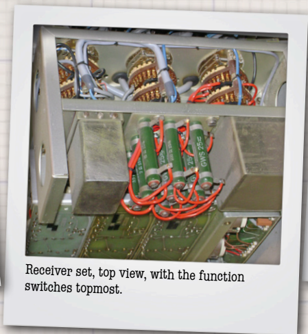
Receiver-set electronics: in the middle, the three hum filters for 50, 100 and 150 Hz.
