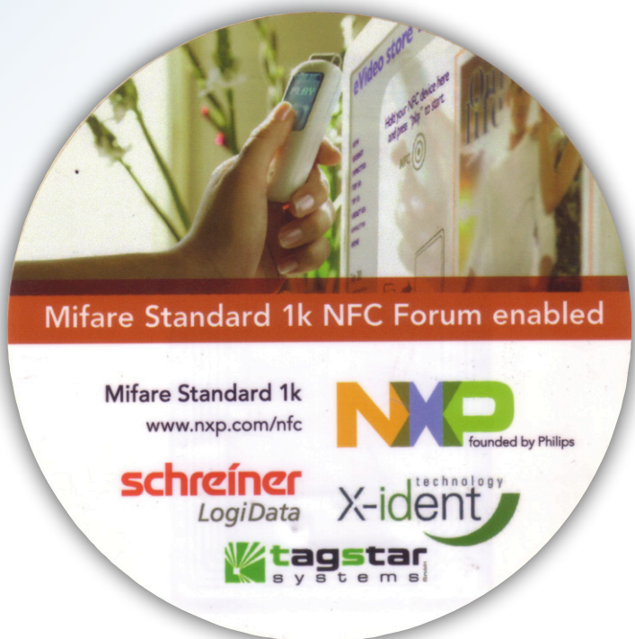
Figure 3. Mifare Classic type tag: 1024 bytes of memory, but limited compatibility.
