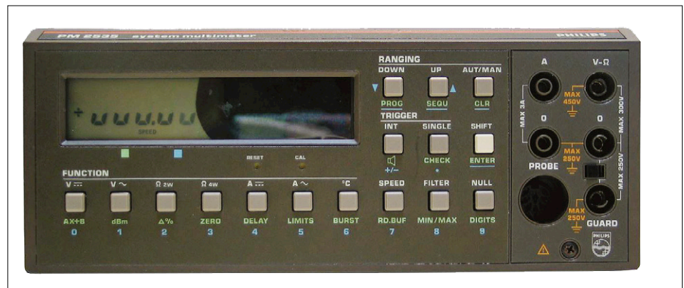
Figure 4. The meter with the defective display, which was beyond repair.
