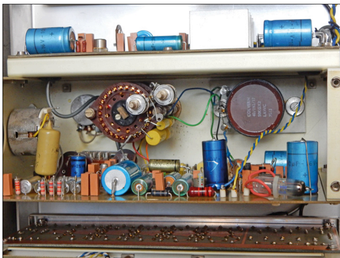
Figure 3. Transmitter set, rear view: the glass tube in the lower-right corner of the board is the thermistor, which is included in the feedback loop.
