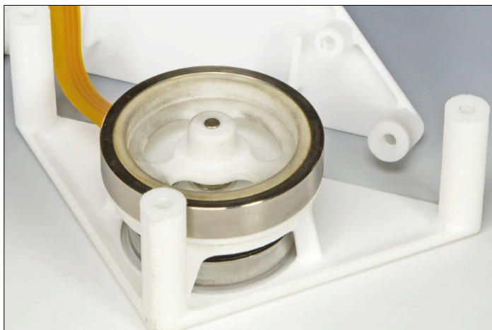
Figure 4. Inertia wheel added to the motor.
