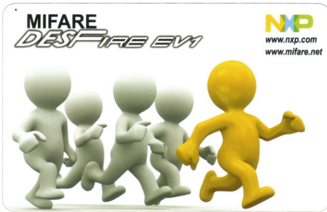
Figure 4. The MIFARE DESFire card from NXP is one of the first “Type 4” tags.
