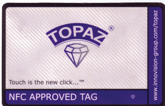
Figure 1. Topaz card from Innovision complying with the NFC Forum "Type 1" specifications.
