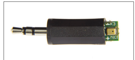
Figure 10. The MEMS microphone can be fitted into the sleeve of a 3.5-mm jack plug.
