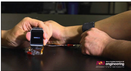
Figure 10. Arizona State University's flexible strap battery is Kirigami-derived.
