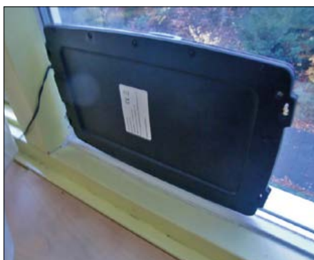
Figure 5. Slow and indirect as it may be in terms of energy transfer, a solar panel and some Dutch sunshine make a fine (and indirect) power source for the charger.
