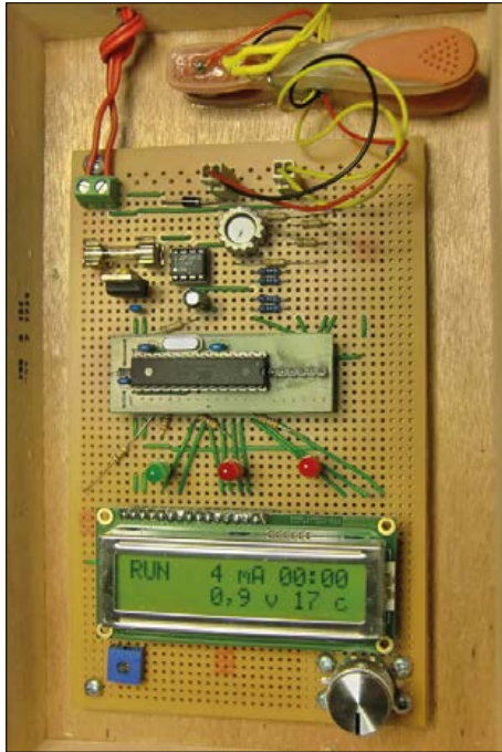
Figure 4. The brains of the project is the ATmega328-based I-Board with its SIL pinheader for plugging onto another board — in this case, a piece of stripboard that's home to the remaining components.
