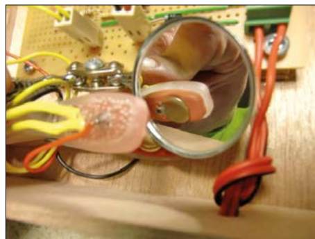
Figure 2. Mirror-aided close up showing the thumbtack contacts on the clothes peg arms.
