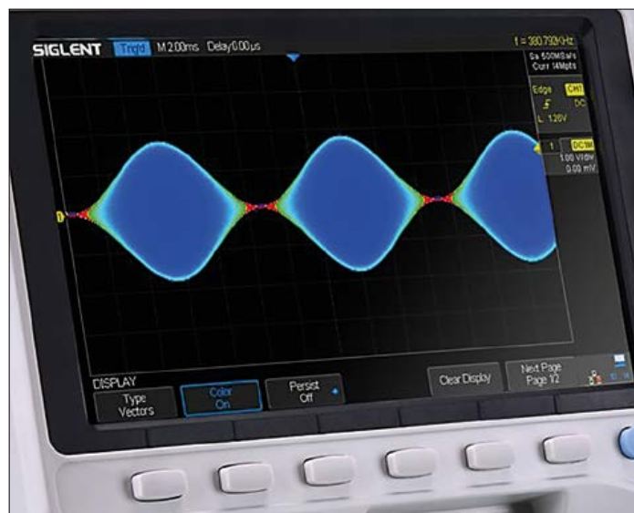
Figure 3. So-called soft keys beside or below the screen are standard on more expensive models too (Photo: Siglent).
