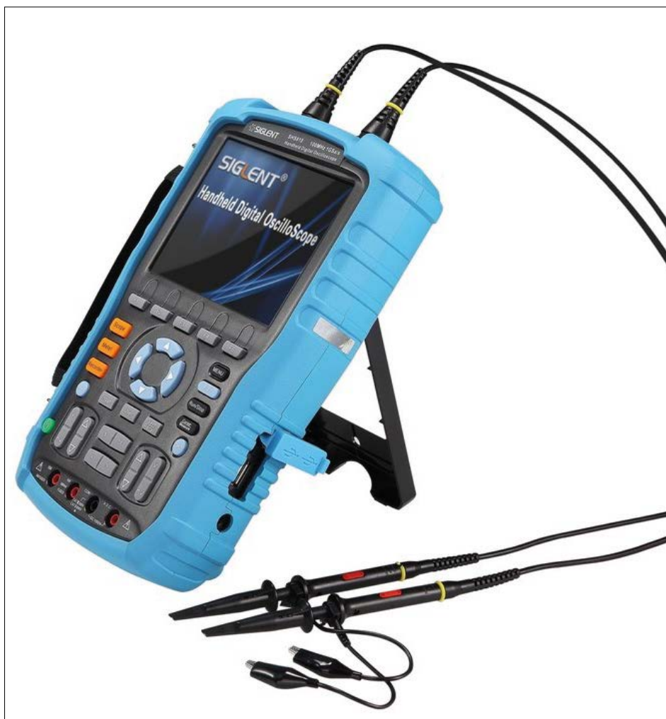
Figure 6. A portable oscilloscope provides all the usual functions in a compact, handheld case (Photo: Siglent).
