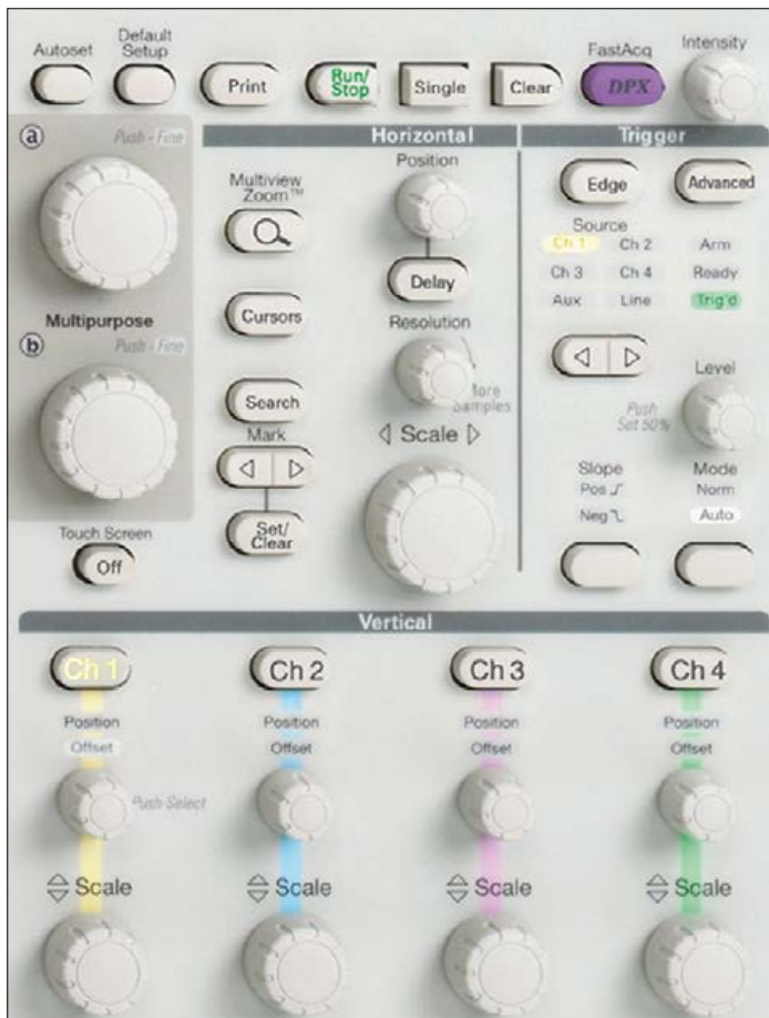
Figure 4. Highly practical: Devices with large front panels provide separate operator controls for each of the channels (Photo: Tektronix).
