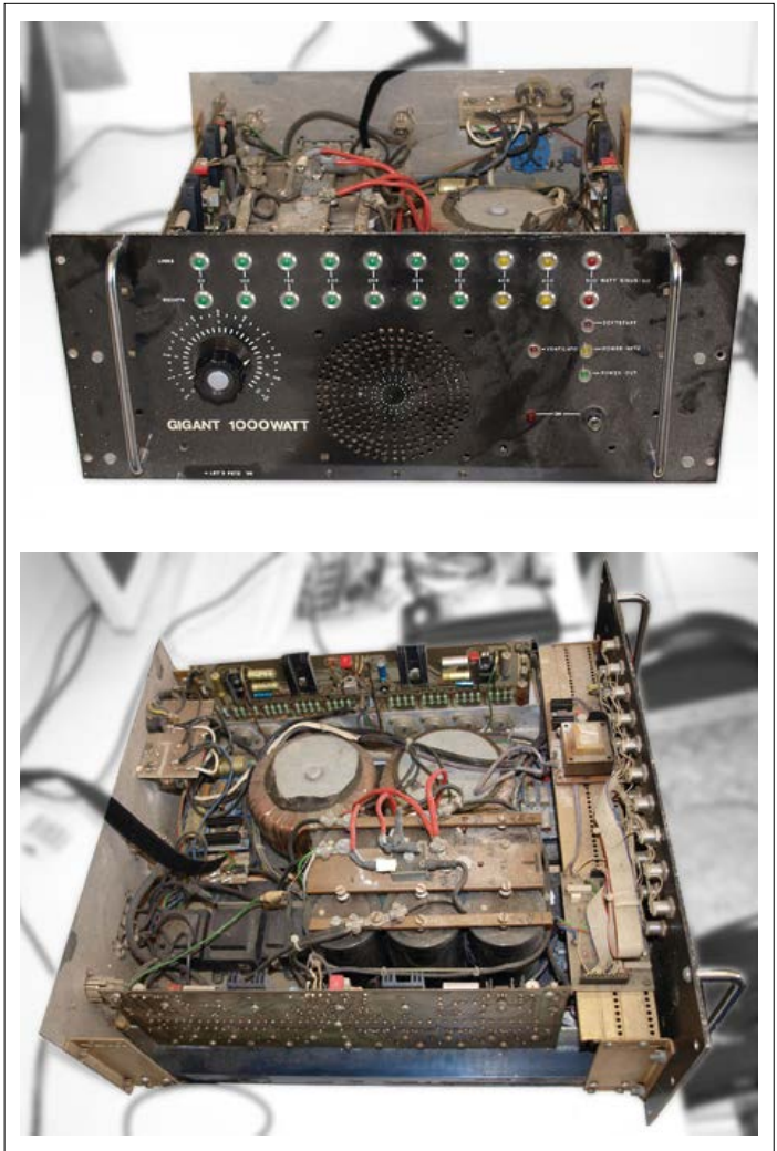
Figure 3. Front view (3a) of Günter Gerold's amplifier with its original 80s patina. His mobile disco rejoiced in the name of 'Let's Fetz!' From above (3b) you can see the effect of pumping thousands of cigarettes' worth of fumes through the unit.
