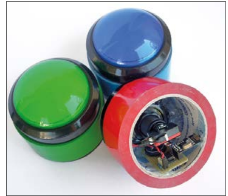
Figure 5. The author's quiz buttons were made from stacked adhesive-tape rolls and industrially rated switches. The housing in different colors is sturdy and has an immediate "Quiz Time" appeal.
