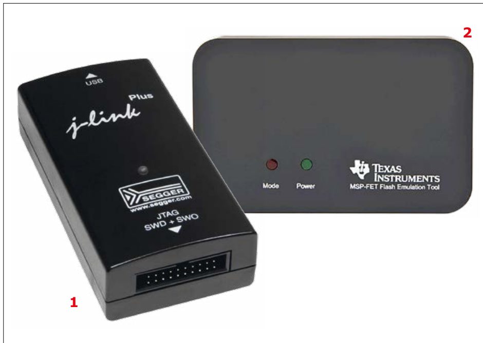
Figure 1. Segger's J-Link for ARM MCUs [1] and the MSP-FET [2] for the MSP430 crowd. Source: Segger/Texas Instruments
