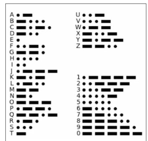
Figure 1. The Morse alphabet or "Wireless Code". Radio telegraphy would be a Tower of Babel without it.
