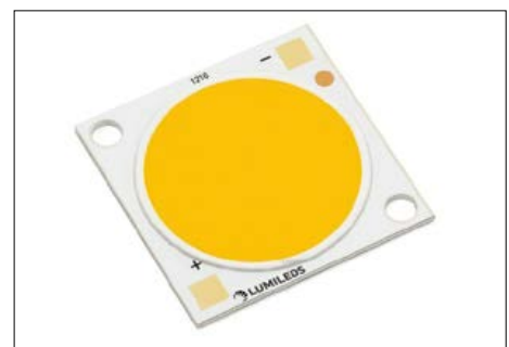
Figure 4. A modern ultra high power LED: the Luxeon CoB 1216. It consists of many blue LEDs mounted on a ceramic substrate and wired in series, all covered by a phosphor layer. This LED produces an astonishing luminous flux of 15,000 lumen.
