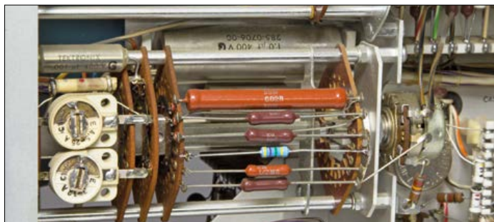
Figure 3. The 5-MΩ 1% tolerance resistor responsible for the “5” positions of the timebase having gone infinite it had to be replaced. A 4.7-MΩ resistor was quickly installed whilst researching the cost of the correct component from Farnell/Newark. I may also decide to fit a 300-kΩ R in series.
