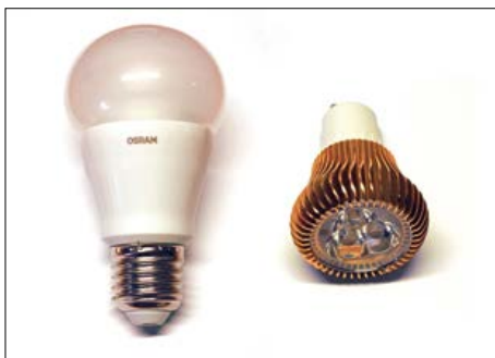
Figure 5. LED lamps are available in every imaginable form with a wide range of color temperatures and versions. Two types are shown here: a 10 W lamp with a conventional form factor and E27 screw base, and a small 4 W spotlight with three LEDs and a GU10 base.
