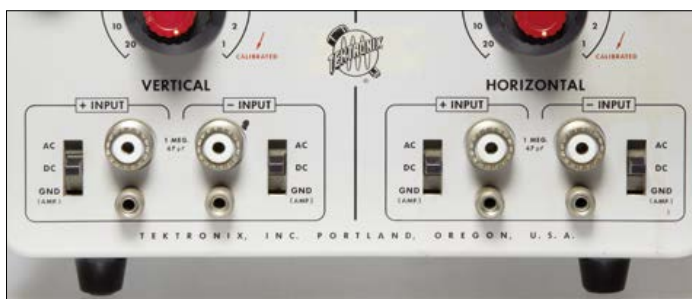
Figure 1. Not too common: an oscilloscope with differential inputs for both Vertical and Horizontal. That’s great for X-Y displaying and for measurements not referenced to ground.
