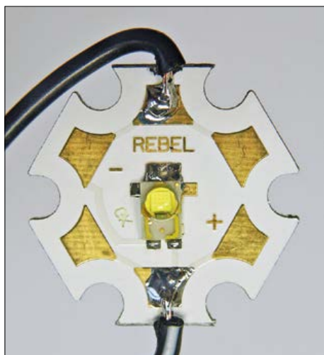
Figure 4. A 3-watt power LED on a circuit board with an aluminum core for heat dissipation.
