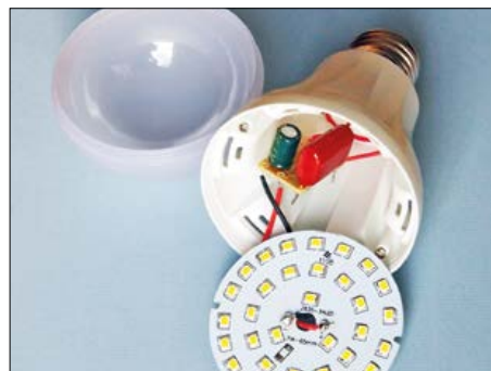
Figure 12. What's inside a cheap LED lamp: a series capacitor, a diode, a filter capacitor and a discharge resistor. The marking on the board says that the rated power is 7 W, instead of the claimed 10 W.
