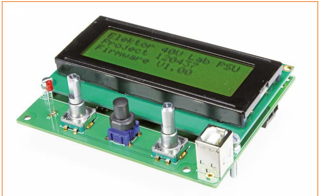
Figure 4. The LCD module is secured to the PCB by a pair of M3 screws and nuts, with extra nuts for the right spacing.
