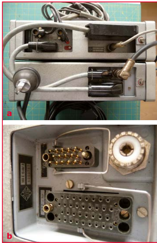
Figure 3. (3a) Cable connections between the S/E 169E15 öbL B radio box and the ancillaries box. (3b) View of the connector bay on the radio box.
