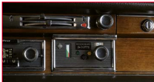
Figure 9. Special version of the carphone control box for the Mercedes W108/W109 dashboard. Merc fans in California, Texas, Florida, Nevada, eat your hearts out. (courtesy and copyright oeb1.de)
