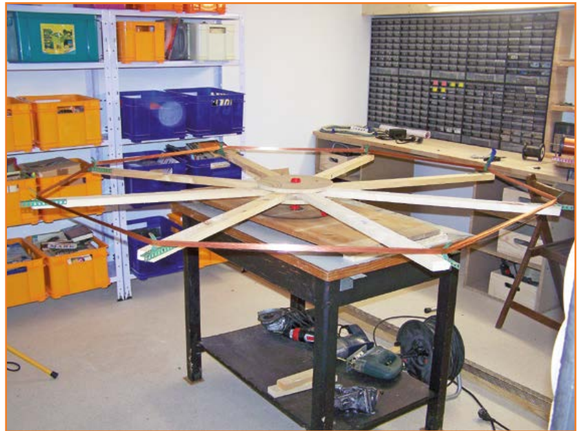
Figure 5. The author's home-made coil winding machine. Smaller versions will suffice for practical applications.
