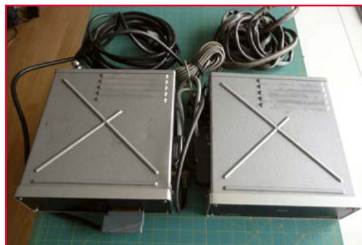
Figure 2. The twin equipment cases of the mobile telephone setup, together with the cable assembly
