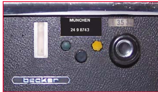
Figure 8. The standard AT400-series "Becker" control box type for dashboard mounting. Still a bit unpolished! (courtesy and copyright oeb1.de)
