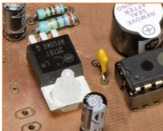
Figure 6. We can see the regulator fitted a small distance from the copper surface.
