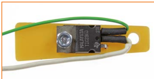
Figure 3. The triac and resistor can easily be mounted inside the soldering iron handle on a small piece of PCB.
