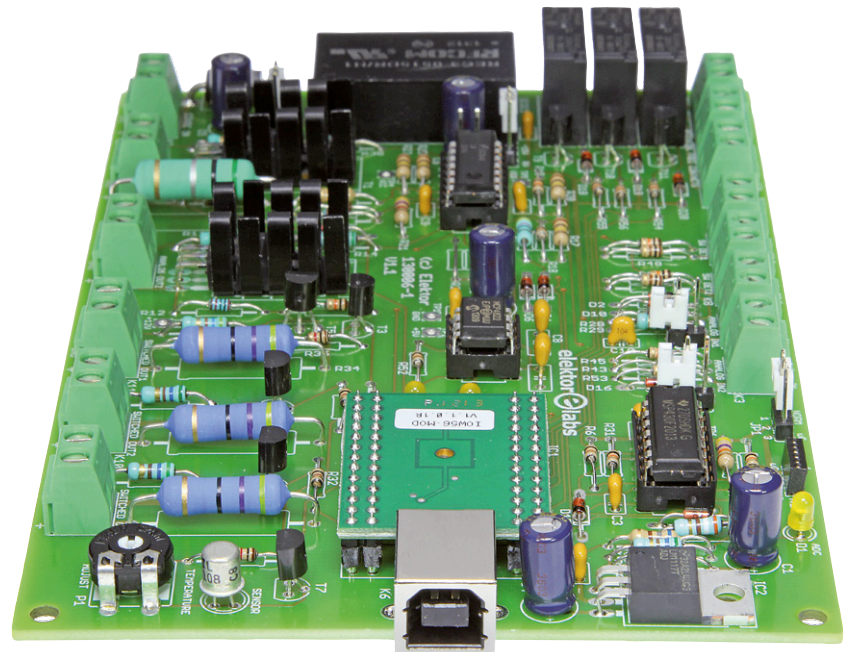
Figure 5. The USB cable is connected directly to the IO-Warrior module.
