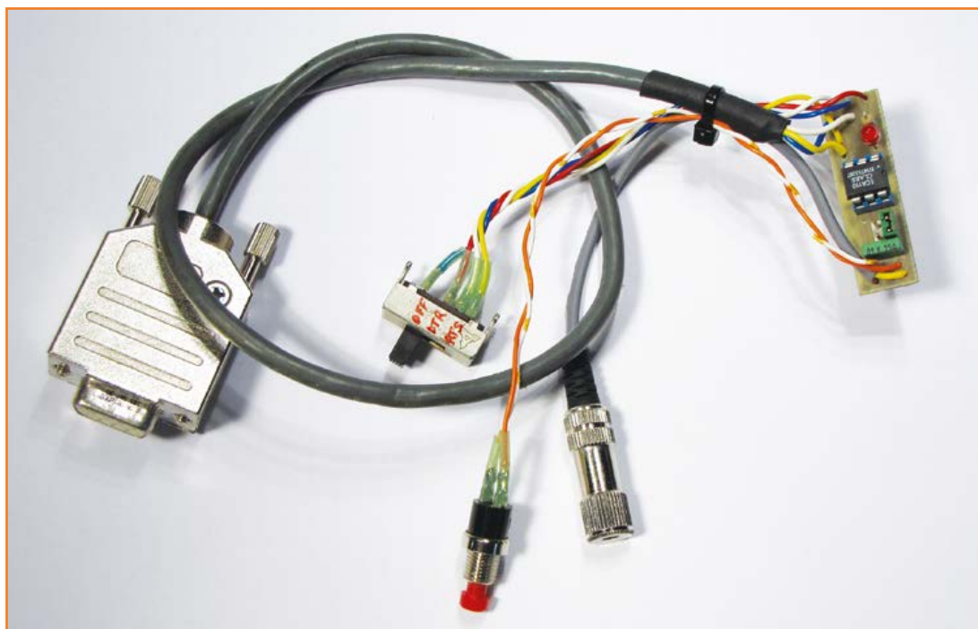
Figure 1. An optocoupler allows us to ensure electrical separation between a PC and the radio it is controlling.
