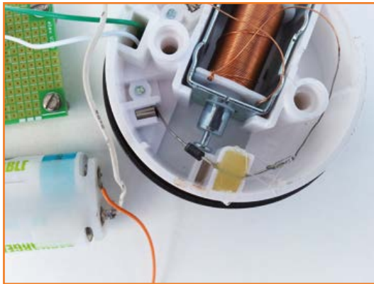
Figure 3. A magnet from a toaster is used here. The flyback diode is connected direct to the inductance.
