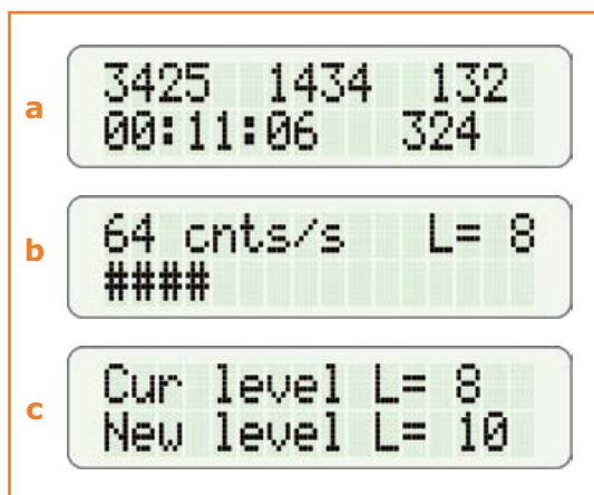
Figure 3. a) Measurement display, b) intensity mode, c) manual setting of the threshold levels.
