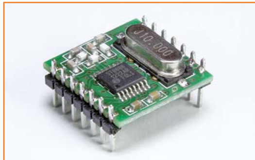
Figure 1. The low-power radio module from Chinese manufacturer HopeRF (433 MHz version shown here with header pins soldered on) is controlled over SPI. Versions are also available for the 868 MHz SRD band.
