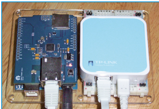
Figure 6. Low-cost Mobile Hot Spots like this TP-Link NanoRouter make it easy to convert Ethernet to Wi-Fi without any software changes.
