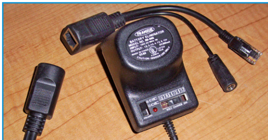
Figure 5. All you need are some cheap 'cheater g' cables (splitter and injector) and a variable power supply to homebrew your own Passive PoE solution.
