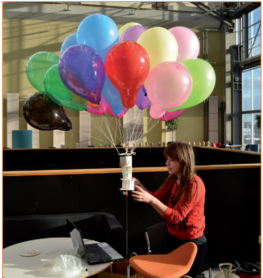
Figure 2. About a dozen balloons appeared enough to lift the Arduino Mobile Weather Station assembly, rather than 25 as initially calculated.
