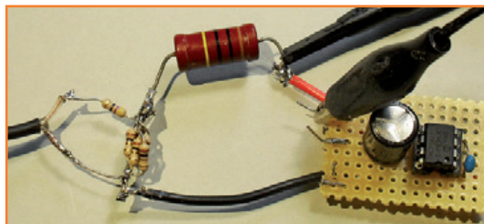
Figure 3. Current measurement with shunt, as in Figure 2.
