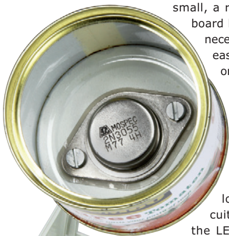
Figure 3. The mounting of the 2N3055 on the bottom of the tin. The transistor still needs to be covered with sealant to make everything waterproof.
