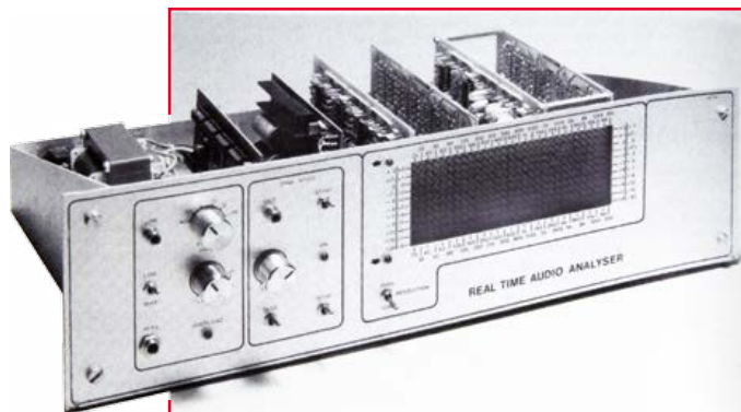
Figure 8. Finished prototype of the Elektor real-time analyser, photographed from an Elektor May 1984 page. (original reproduction by copyright holder)
