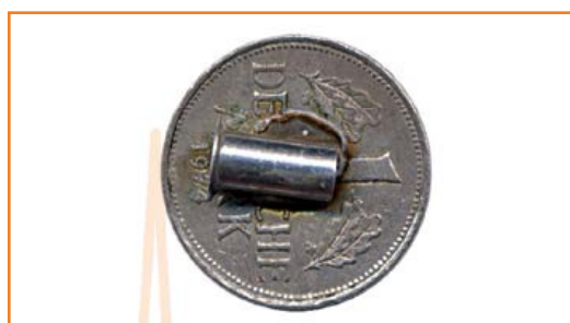
Figure 30. Satisfactory electrodes can be obtained using nickel-silver coins, as long as you can manage to solder to them a 4-banana socket.
