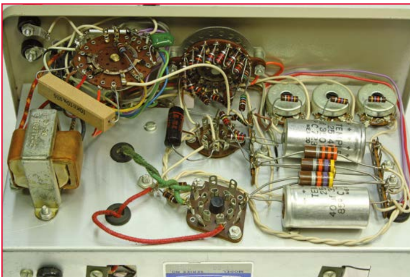
Figure 6. A view of the component side of the chassis. The leftmost wafer is the Bridge/Discharge/Leakage switch. The middle wafer switch is the voltage ladder for selecting the working voltage. The three potentiometers in the upper right adjust the leakage threshold for each capacitor type.
