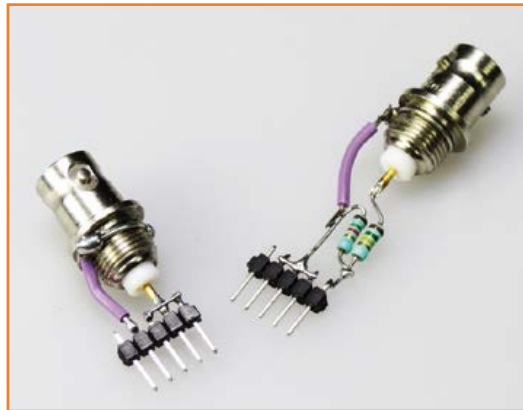
Figure 23. You'll only need to turn on your soldering iron to build these two calibration jigs.
