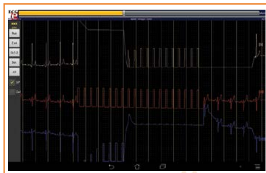
Figure 27. Every minute, the interface produces a 2 Hz/1 mV CAL signal for 10 s, which can be used for balancing the gains (see Figure 26).
