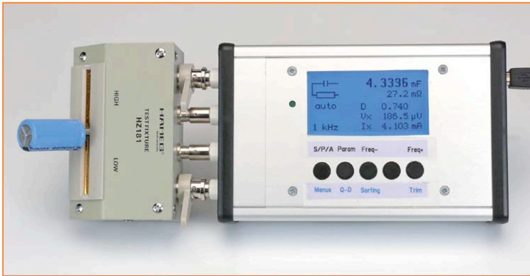
Figure 7b. This test fixture fitted directly to the LCR meter case can be found for around $50.
