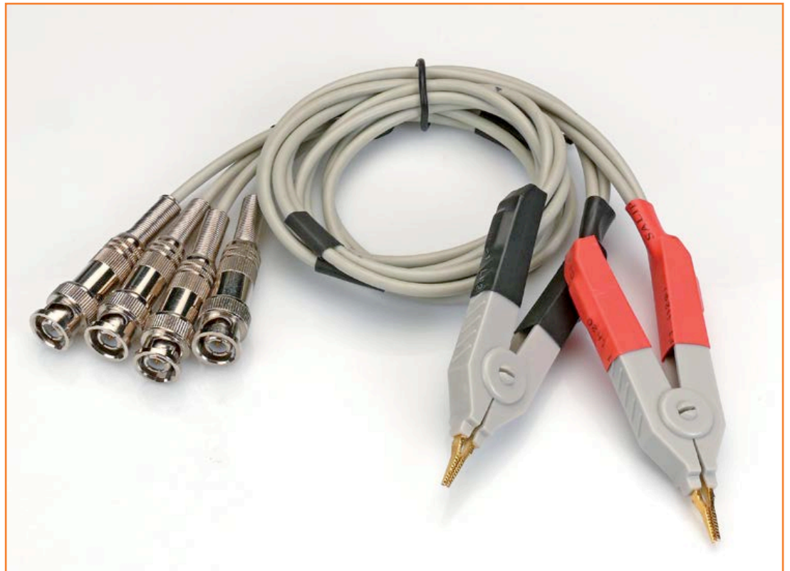
Figure 7a. This set of Kelvin clips with four BNC leads can be found for around $10.
