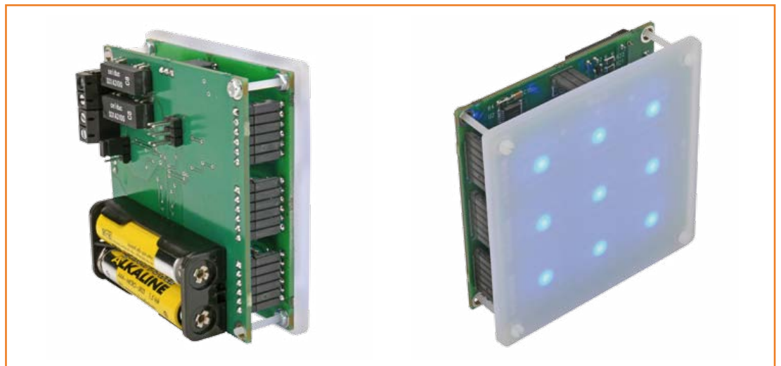
Figure 10. To ease the mounting of the sheet onto the keypad, solder the connectors from the underside so they do not protrude.
