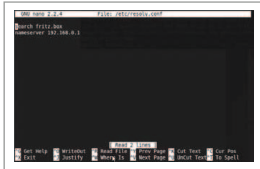
Figure 4. Configuration of the DNS server.
