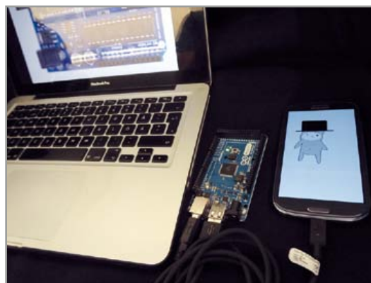
Figure 2. Arduino Mega ADK connected to a PC and to a phone.
