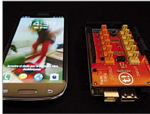
Figure 1. Arduino Mega ADK with Tinker Kit Shield and phone.
