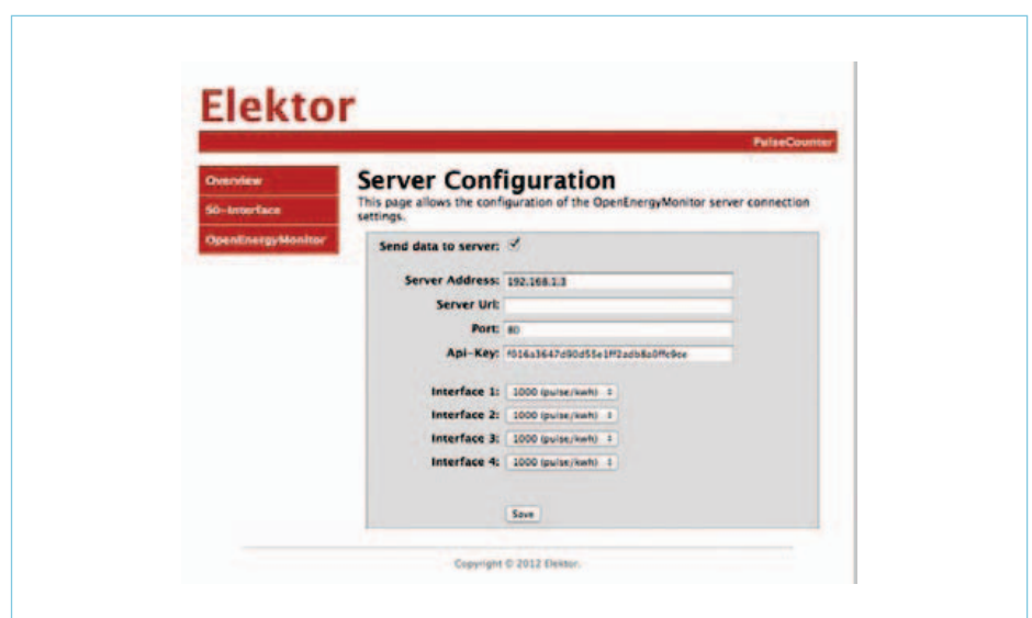
Figure 4. OpenEnergyMonitor server configuration.
