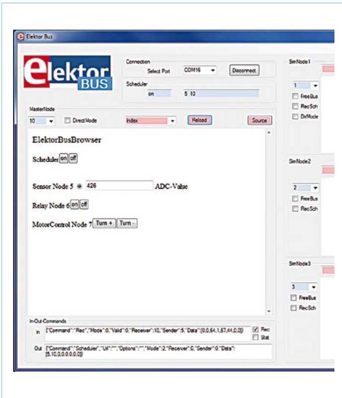
Figure 5. A very simple HTML user interface for trying out the three example applications.
