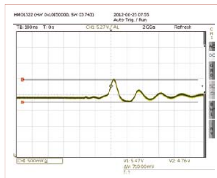
Figure 6. Response to pulsed load.
