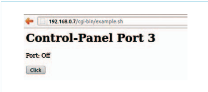
Figure 14. LED switching in the browser.
