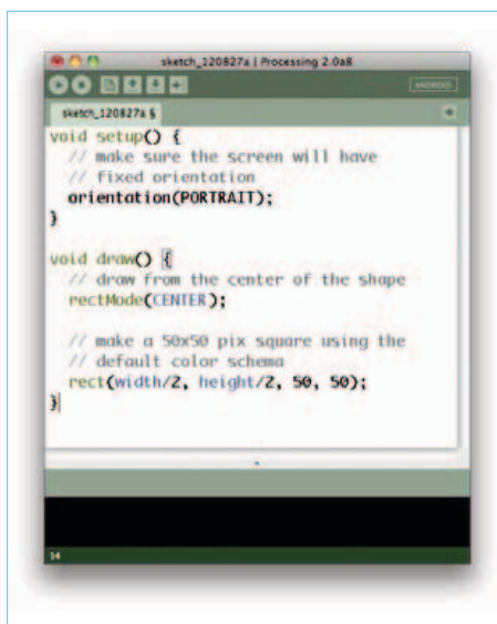
Figure 8. Screenshot of Processing running Android mode; note the Mode button in the upper right corner.
