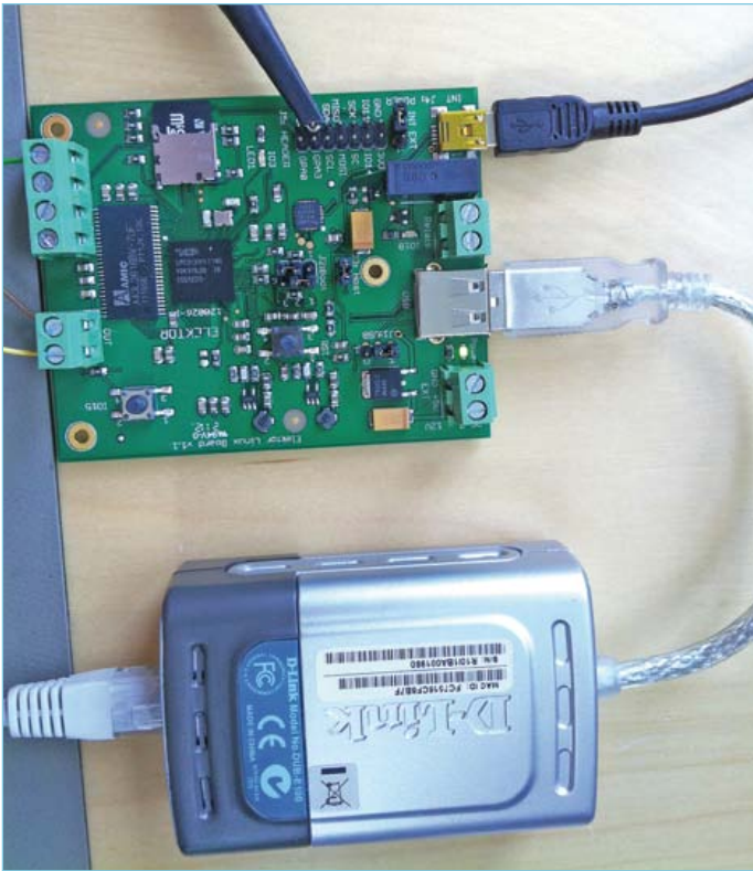
Figure 9. A USB/LAN adapter gives the board a network interface.
