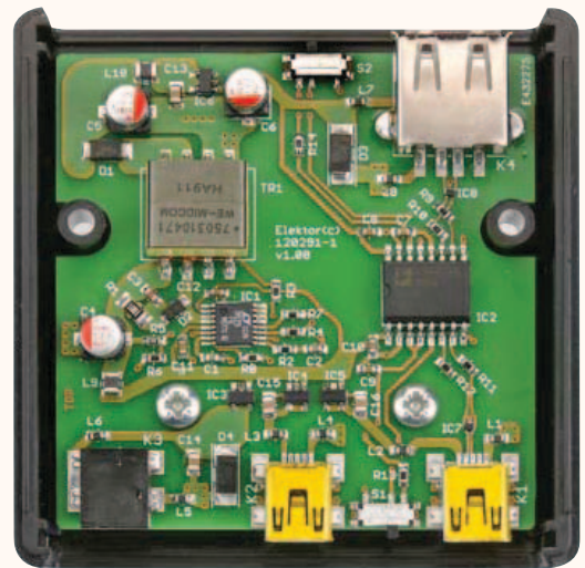
Figure 3. The dimensions of the board were chosen to fit in a type 1593KBK case from Hammond.
