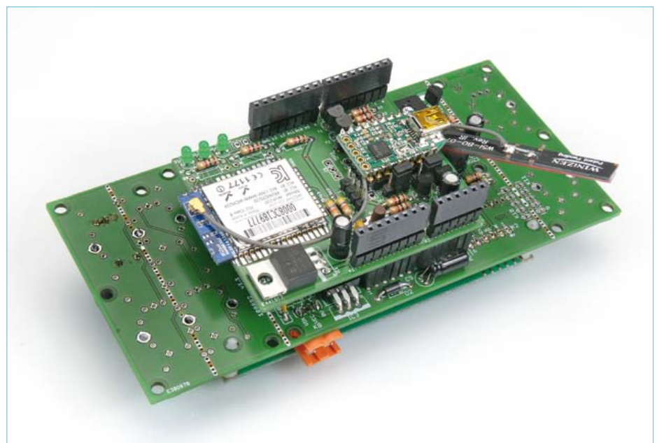
Figure 2. Fully built-up Wi-Fi shield on top of Platino, also equipped with a 20x4 alphanumerical LCD.
