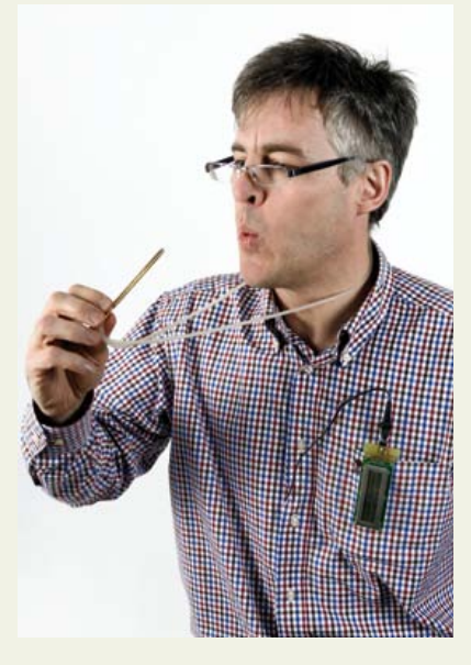
Figure 10. For the calibration, make sure you place the Pitot tube inlet at exactly the same height as the thermistors, so that the air-flow is the same for both anemometers.
