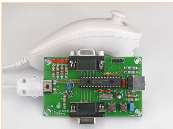
Figure 6. The two slots made with a min disc-cutter are vital so as to be able to plug the controller cable in.
