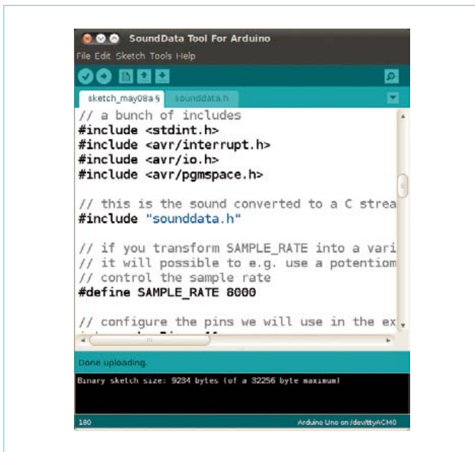
Figure 5. Screenshot of the basic sound player after automatically generating the code.
