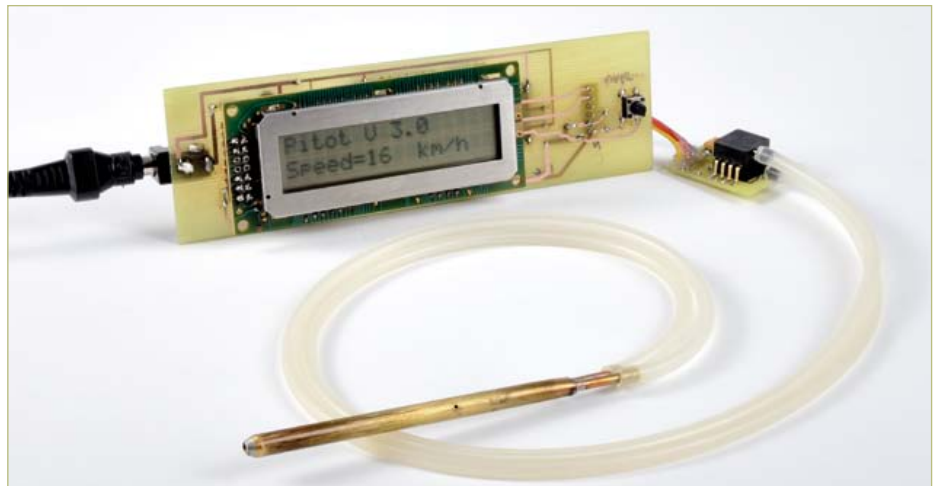
Figure 4. The second prototype for my Pitot tube anemometer.
