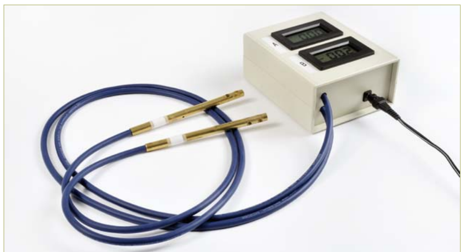
Figure 6. My prototype for the dual hot-wire anemometer for dual-flow ventilation, with its two probes and the corresponding displays.
