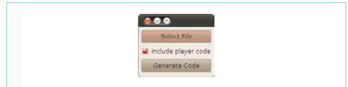
Figure 3. Dialog Window to import WAV files into your Arduino sketches as header files.
