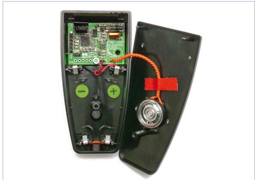
Figure 7. My prototype. The magnetometer is extremely sensitive and is affected by the speaker's permanent magnet. I kept them as far apart as possible, otherwise the total saturation of the magnetometer would have prevented any valid measurements. In spite of everything, the permanent magnetic field from the L/S magnet received by the detector is relatively high, but the compensation algorithm makes it possible to cancel out the effects.
